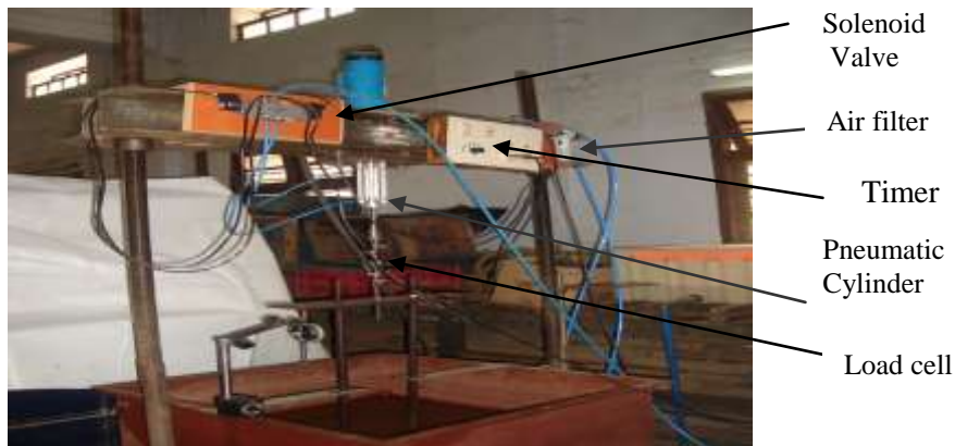
Plate 1: Test set up for monotonic and cyclic loads
