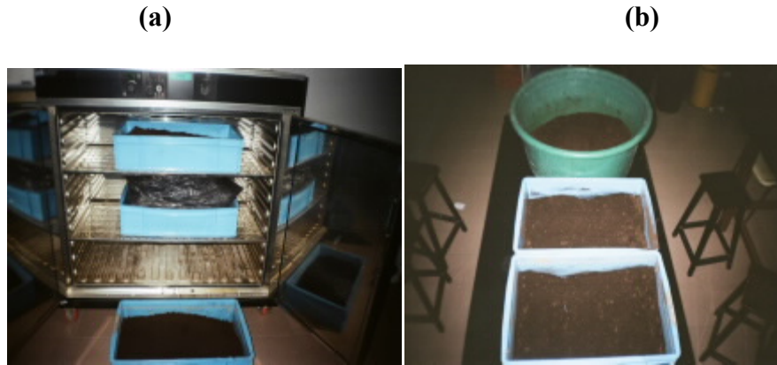
Figure 3: (a) Gradual moisture content reduction or half drying of peat soil procedure in the oven for compaction tests, (b) Reduced moisture content samples to be used for compaction tests.
