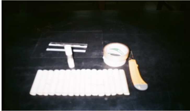
Figure 4: Non-reusable molds (plastic tubes) for columns made of plastic sheet cover and tape
