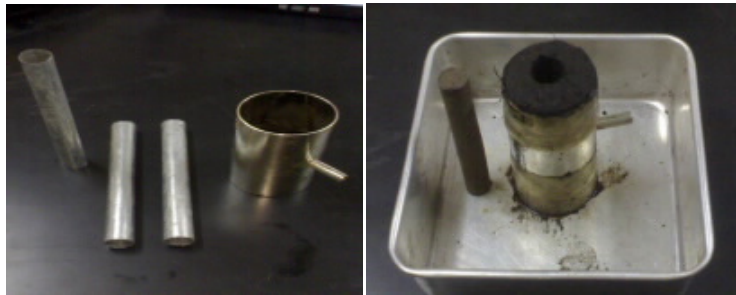
Figure 5: (a) Thin-walled metal tube cutters used to make hole at the center of undisturbed peat soils. (b) Precast stabilized peat column to be inserted in the center of triaxial undisturbed peat soil sample.
