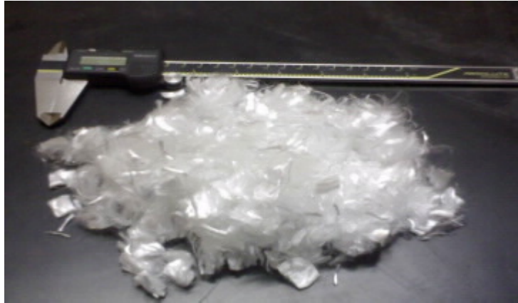
Figure 1: About 50 grams of the type of polypropylene fibers used in the research.
