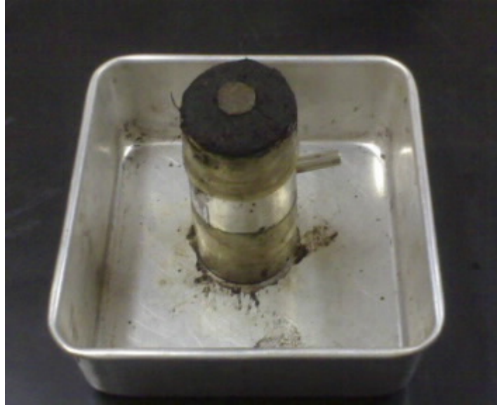
Figure 6: Triaxial undisturbed sample with the precast stabilized peat column placed at its center.
