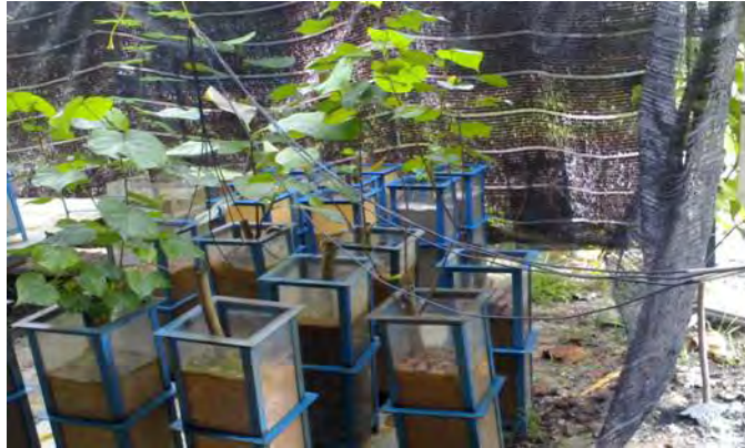
Figure 21: Samples for soil suction testing beside the shade-house
