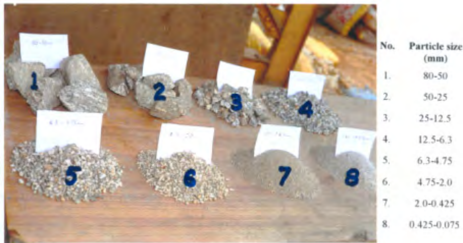
Figure 2: Purulia Dam Materials
