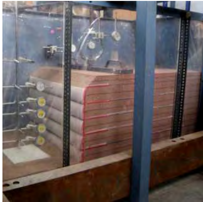
Figure 2: Test setup for wrap-around reinforced soil wall
