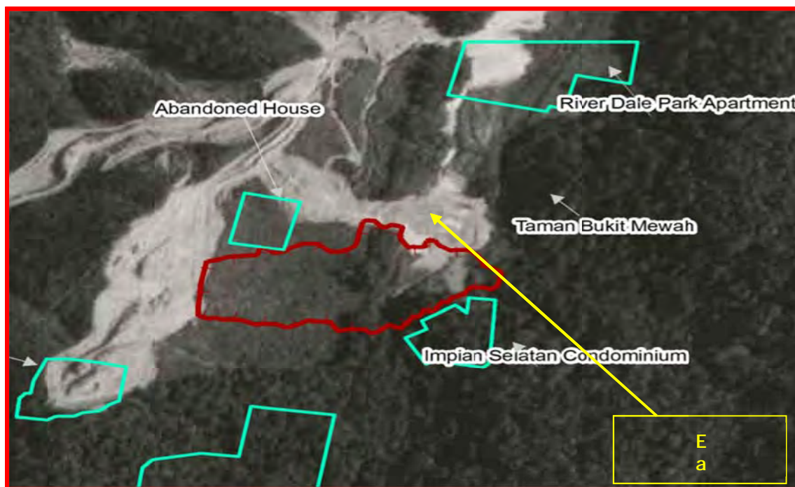
Figure 4: Aerial photograph (1975 by Department of Surveying and Mapping Malaysia) showing evidence of Earth Dumping
