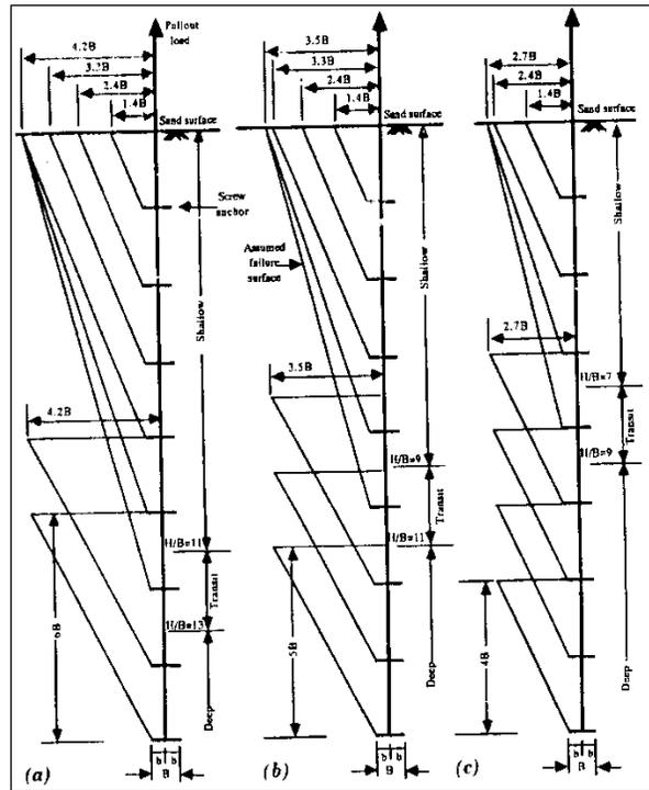
**Figure 12:** Assumed Failure Surface (a) Dense Sand; (b) Medium Dense Sand
