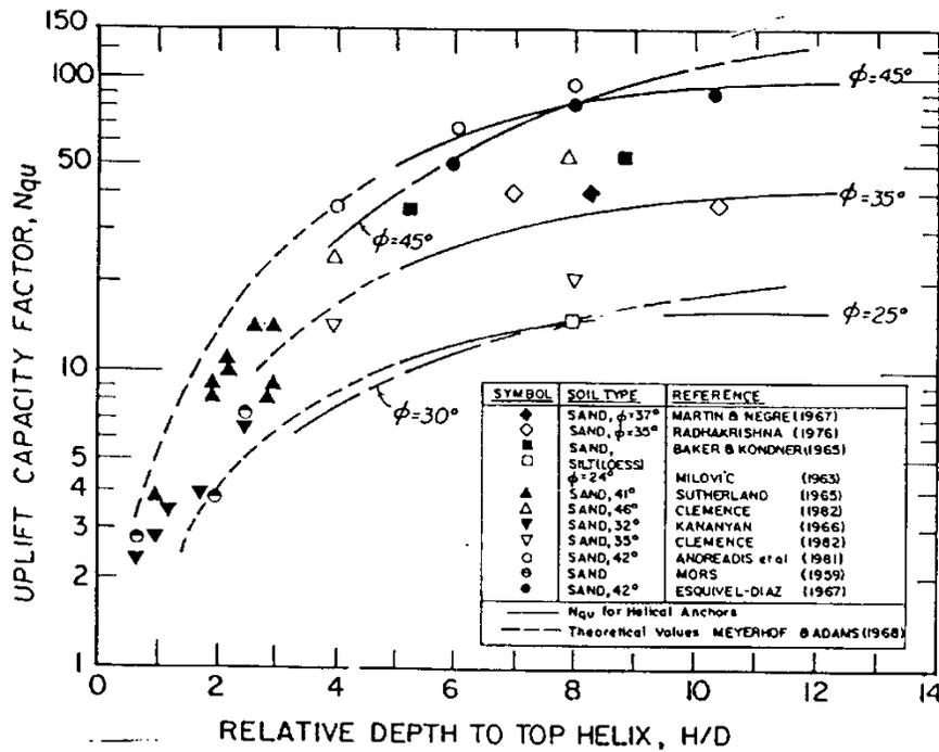
Figure 5: Plot of Breakout Factor with Embedment Depth Ratio (Mitsch and Clemence, 1985)
