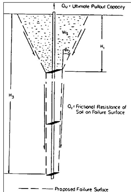
**Figure 7:** Failure Surface of Shallow Helical Anchor in Sand (Mitsch and Clemence, 1985)
