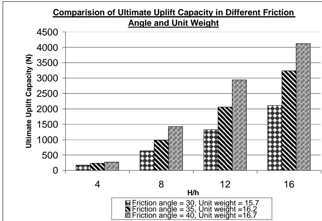
**Figure 6:** Comparison of Ultimate Uplift Capacity in Different Soil Characteristics (Ghaly et. al, 1991 –Table 2 and 3)
