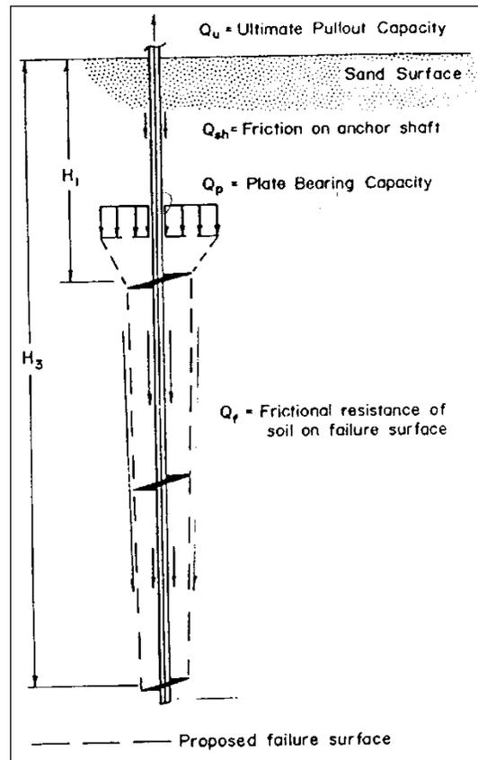
**Figure 8:** Failure Surface for Deep Helical Anchor in Sand (Mitsch and Clemence, 1985)
