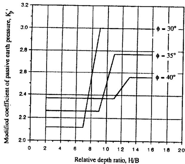
**Figure 13:** Relationship of Modified Coefficient of Passive Earth Pressure and Relative Depth Ratio
