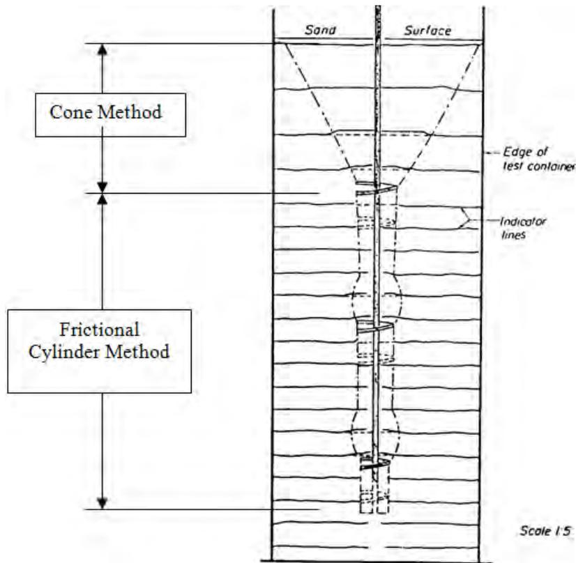
**Figure 3:** Cone Method and Friction Cylinder Method (Mitsch and Clemence, 1985)
