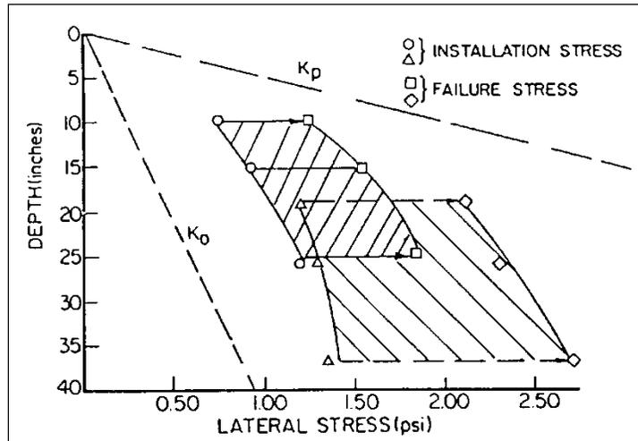
**Figure 9:** Lateral Stress versus Depth for Anchor Installation and Pullout in Medium Dense Sand (Mitsch and Clemence, 1985)
