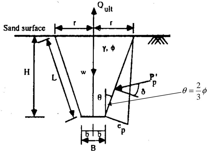
**Figure 2:** Cone Shape Failure Surface (Ghaly et al., 1991)
