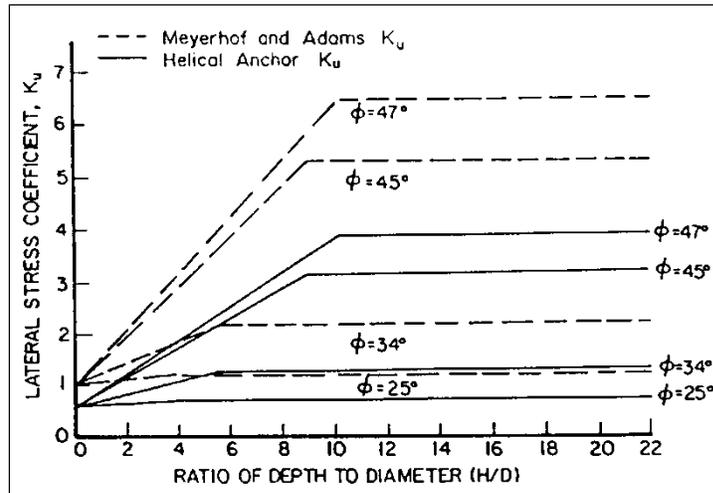
**Figure 10:** Recommended Lateral Stress Values ( $K_u$ ) for Helical Anchors (Mitsch and Clemence, 1985)
