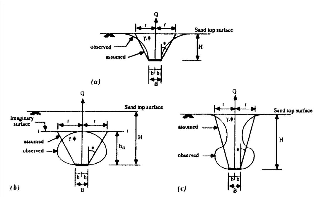
**Figure 11:** Failure Surface for (a) Shallow Helical Anchor; (b) Transit Helical Anchor (c) Deep Helical Anchor (Ghaly et. al, 1991)
