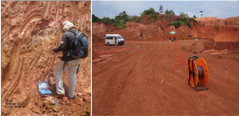
**Figure 1:** Induced polarization (IP) tester meter (left) and IP survey used in this study (right)
