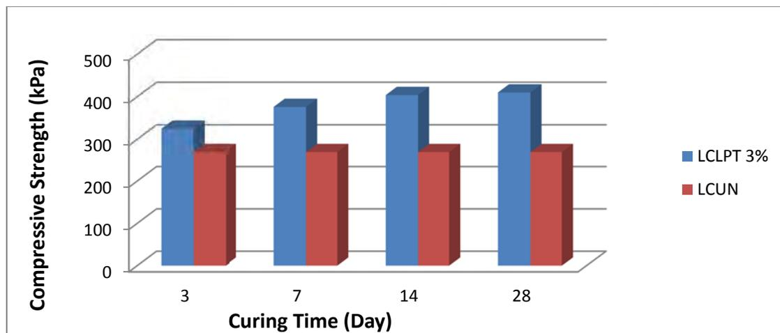
**Figure 4:** Variation of unconfined compressive strength of samples with curing time
