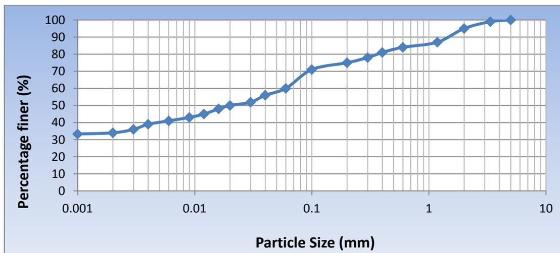
**Figure 1: Particle Size Distribution**
