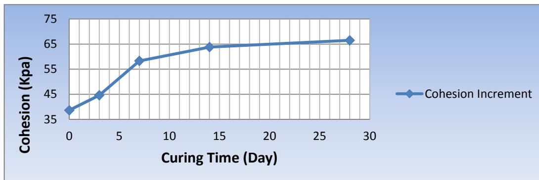
**Figure 10:** Cohesion Increment of Soil by added 9% of SS299
