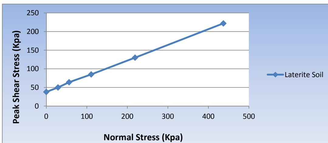
**Figure 9:** Peak Shear Stress-Normal Stress curve for Laterite Soil
