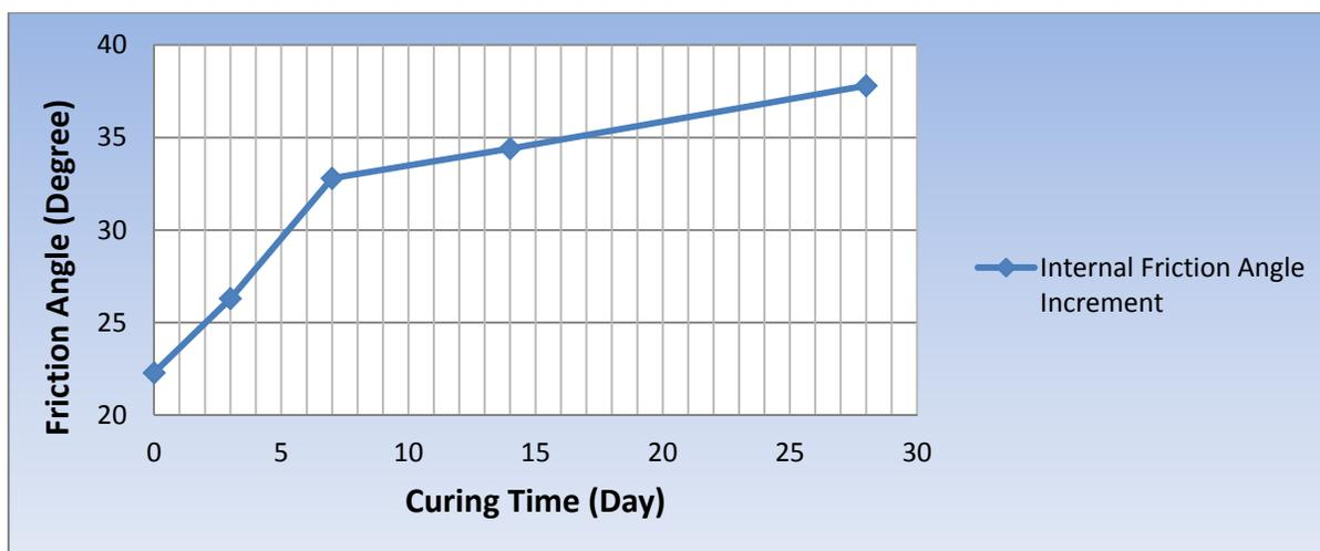
**Figure 11:** Internal Friction Angle Increment of Soil by added 9% of SS299
