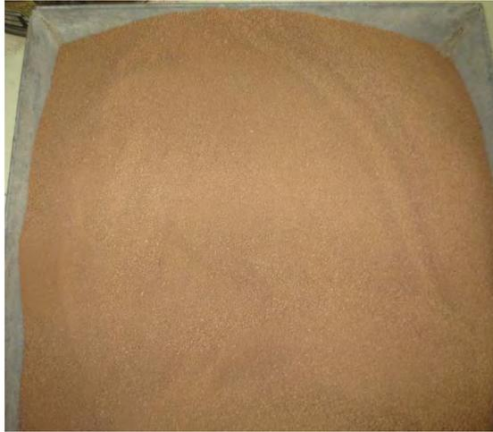
**Figure 2:** Air- dried Laterite Soil
