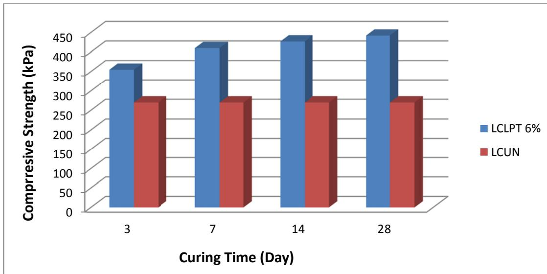
**Figure 5:** Variation of unconfined compressive strength of samples with curing time
