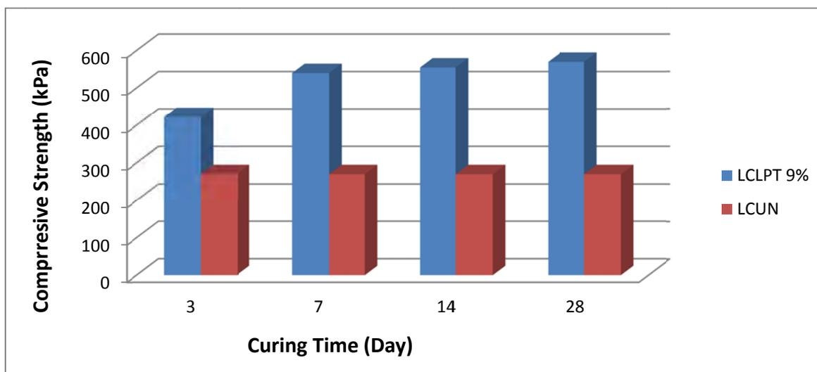
**Figure 6:** Variation of unconfined compressive strength of samples with curing time
