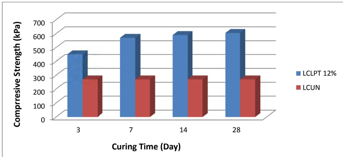
**Figure 7:** Variation of unconfined compressive strength of samples with curing time
