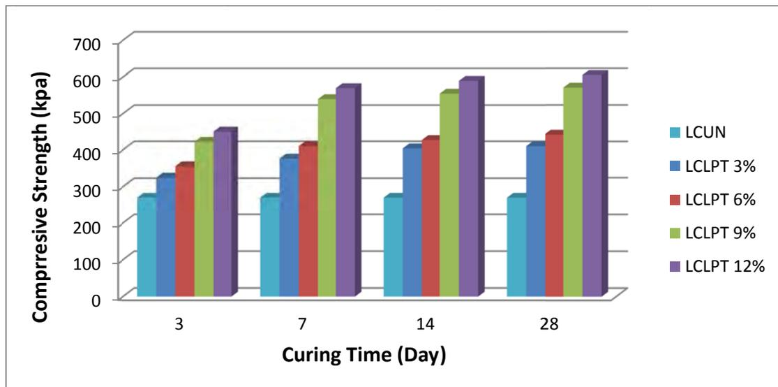
**Figure 8:** Comparison of unconfined compressive strength of samples with curing time
