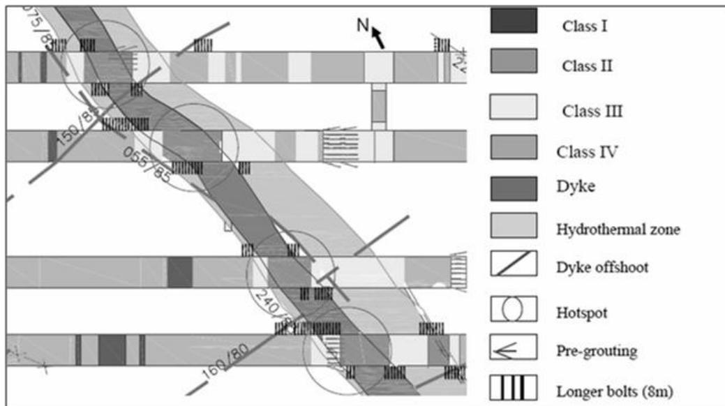
**Figure 5:** Hot spot location and rock mass classification
