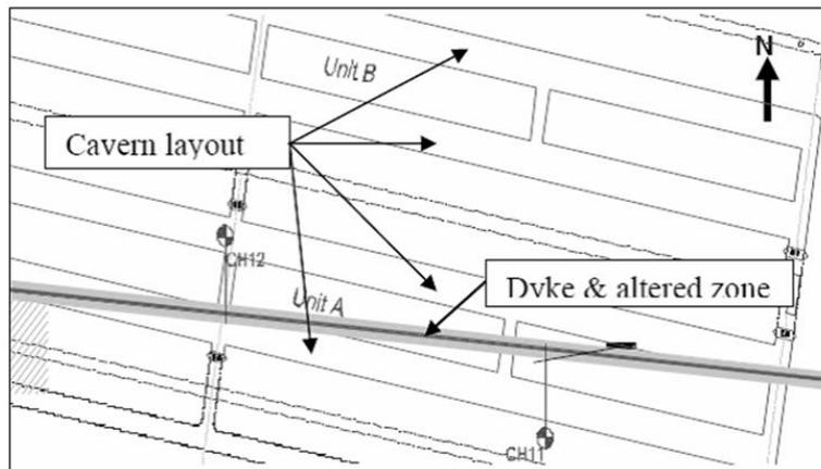
**Figure 2:** 2D Geological model of the storage area showing borehole and geological features
