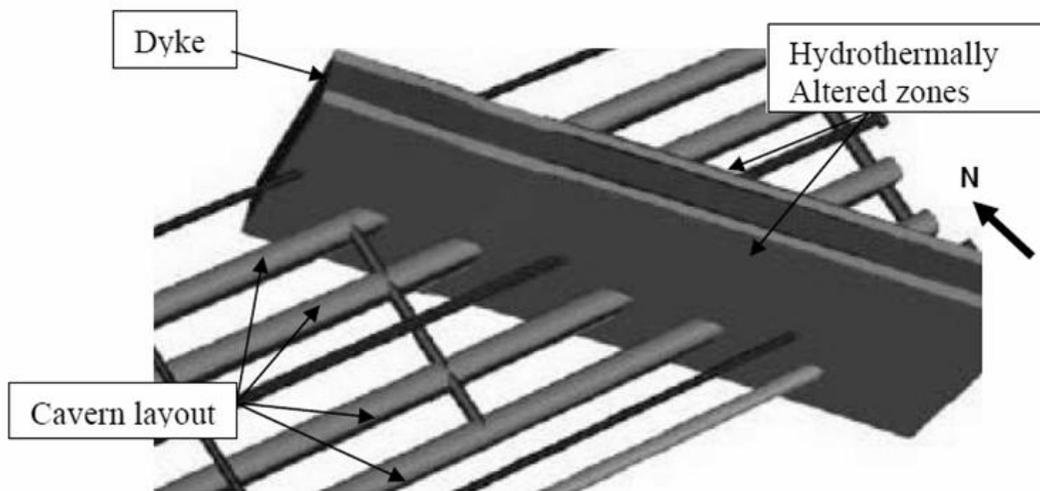
**Figure 4:** Dyke along with hydrothermal zones intruding storage caverns
