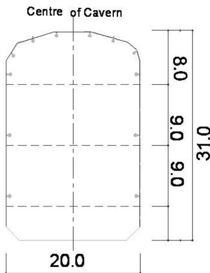
**Figure 7:** Optical targets located in caverns
