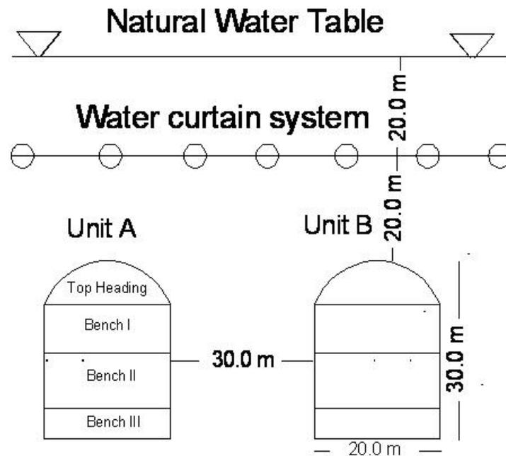
**Figure 3:** Cross-section of storage units along with water curtain system
