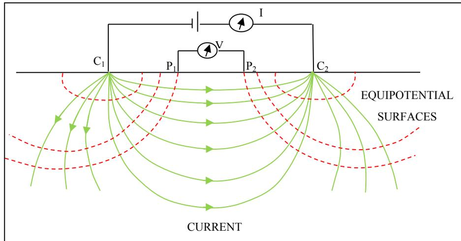
**Figure 2:** Four-point electrode configuration in a two-layer model of resistivity,  $\rho_1$  and  $\rho_2$ . I, current; U, voltage; C, current electrode; P, potential electrode (Modified from Said, 2007).
