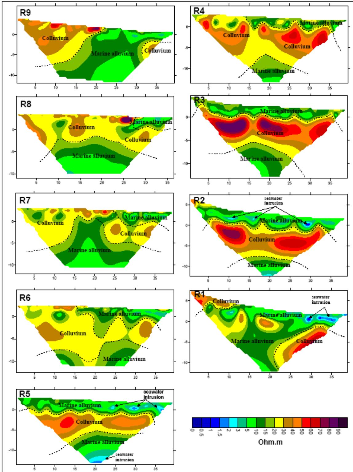
Figure 4: 2-D resistivity inversion model of R1-R9.
