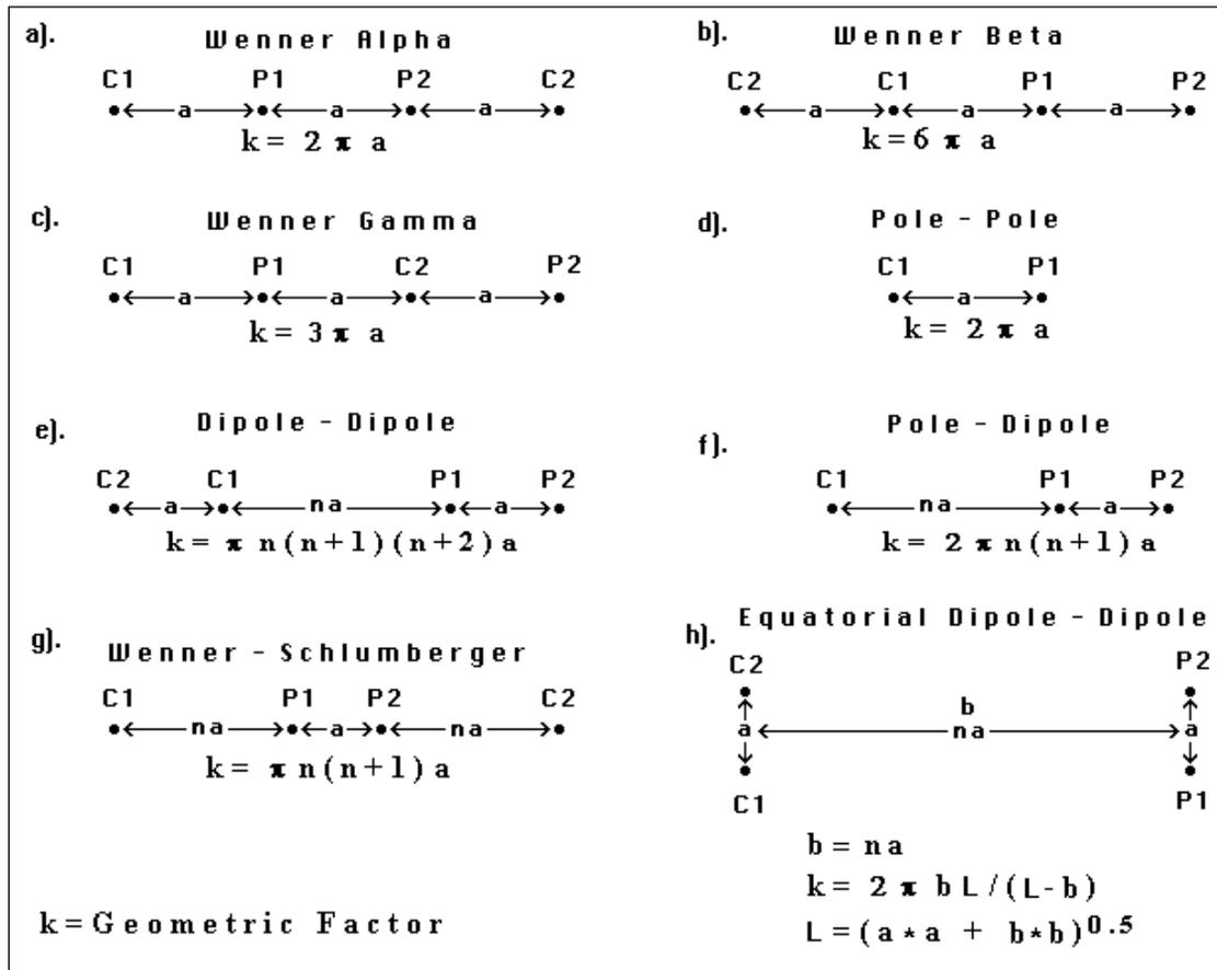
**Figure 3:** Common array for 2-D resistivity measurement (Loke and Barker, 1996)
