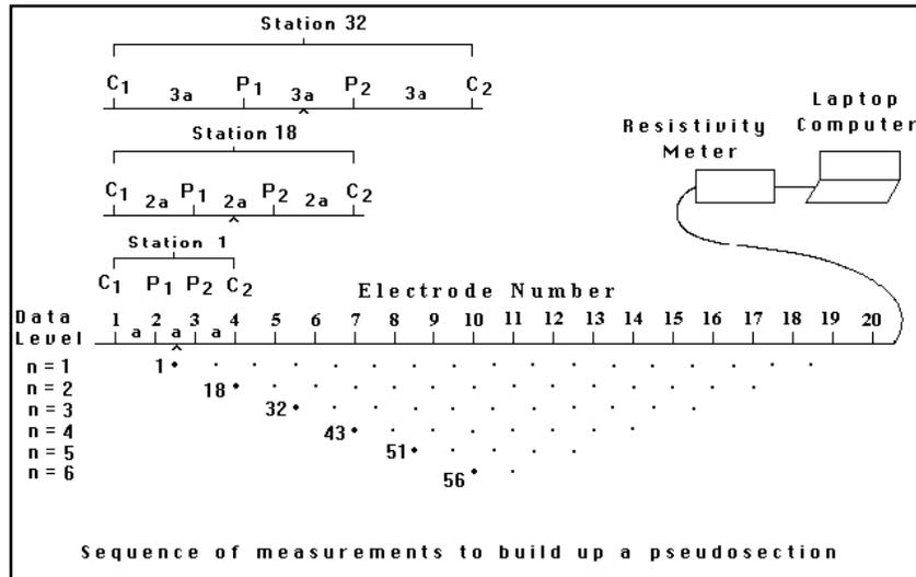
**Figure 3:** The arrangement of electrodes for a 2-D electrical survey and the sequence of measurements used to build up a pseudo section (Loke, 1997).
