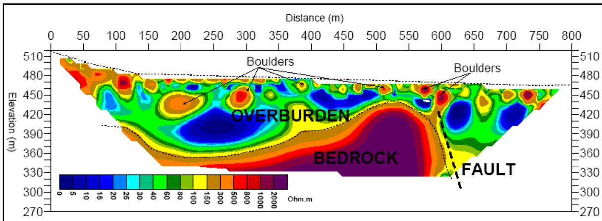
**Figure 5:** Final pseudo-section model of 2-D resistivity survey line at Tangse.
