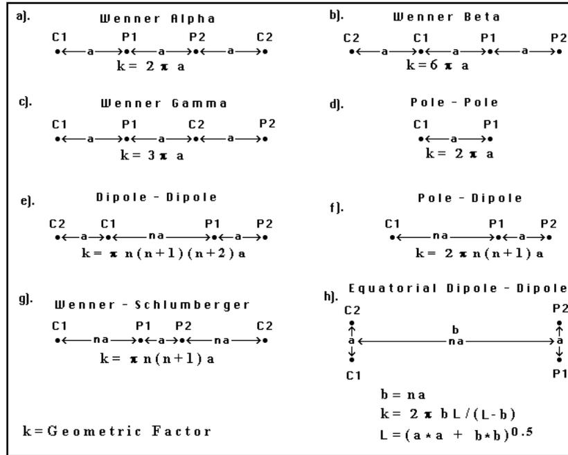
**Figure 4:** Common arrays used in 2-D resistivity surveys and their geometric factors (Loke and Barker, 1996a).
