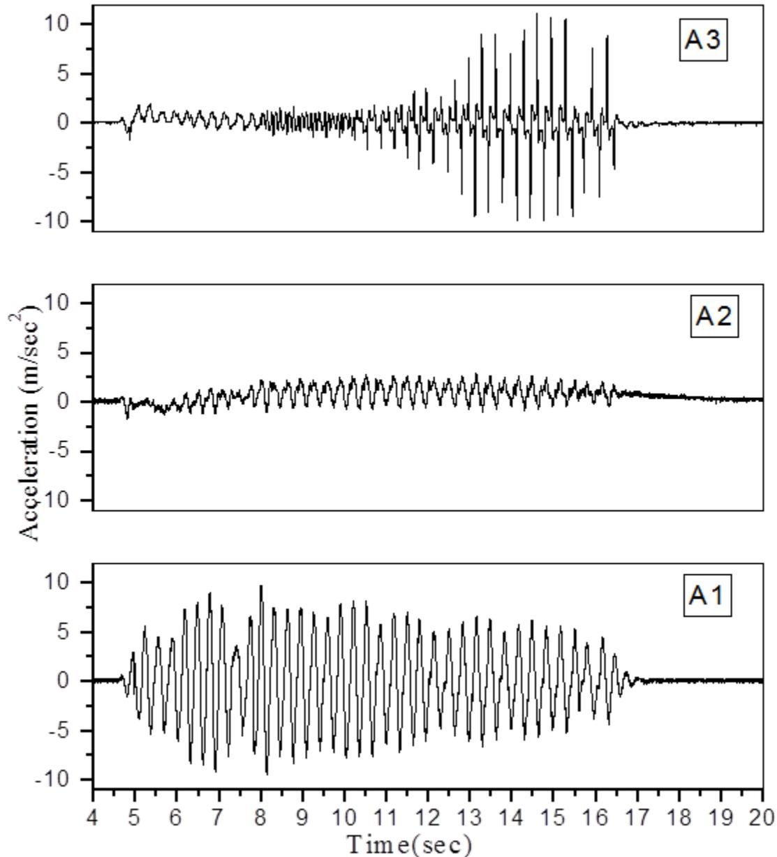
**Figure 6:** Acceleration time histories in shaking table test [1].
