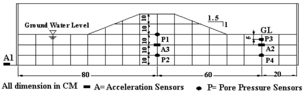
Figure 3: Position of transducer [1]
