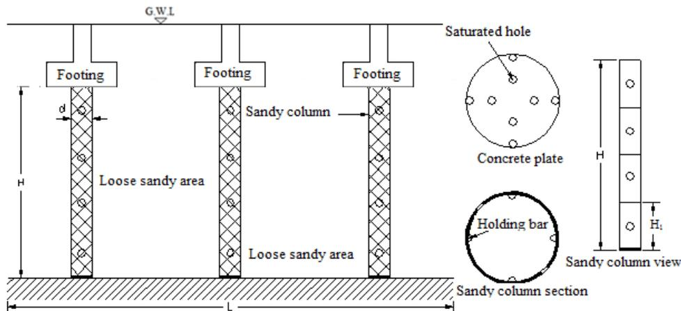
**Figure 2:** Sandy saturated semi-confined columns used under footing for improving light structure stability
