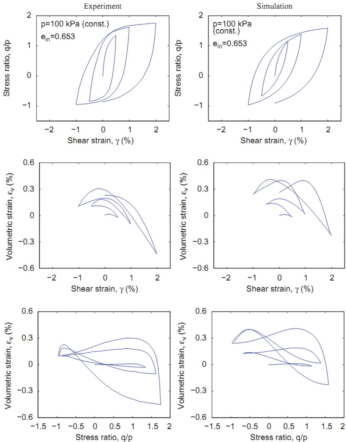
**Figure 1:** Simulation vs. experiments in constant-p cyclic triaxial tests on a relatively dense sample of Toyoura sand [40].
