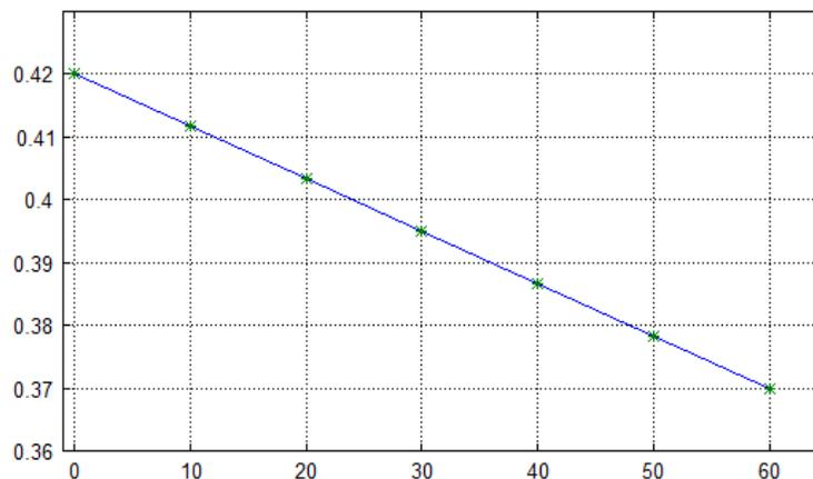
**Figure 4:** Poisson's ratio of liquefied soil from A3 to A2, during subjected to dynamic force
