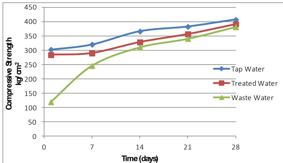
**Figure 5:** Compressive strength of concrete cubes.
