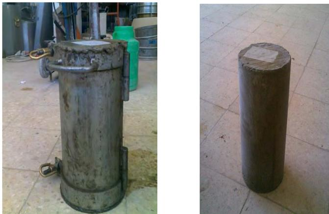
**Figure 3:** prepared cylinder sample
