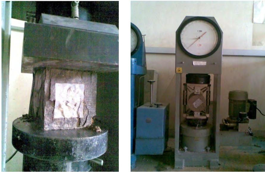
**Figure 4:** The compression and splitting machines respectively
