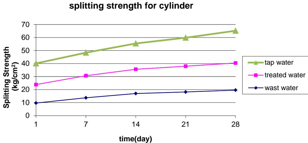
**Figure 6:** Splitting strength of concrete cylinder
