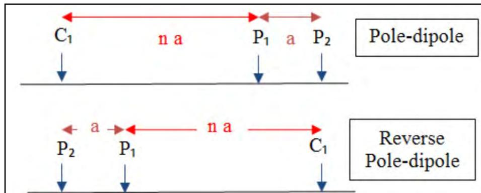
**Figure 3:** The forward and reverse pole-dipole array
