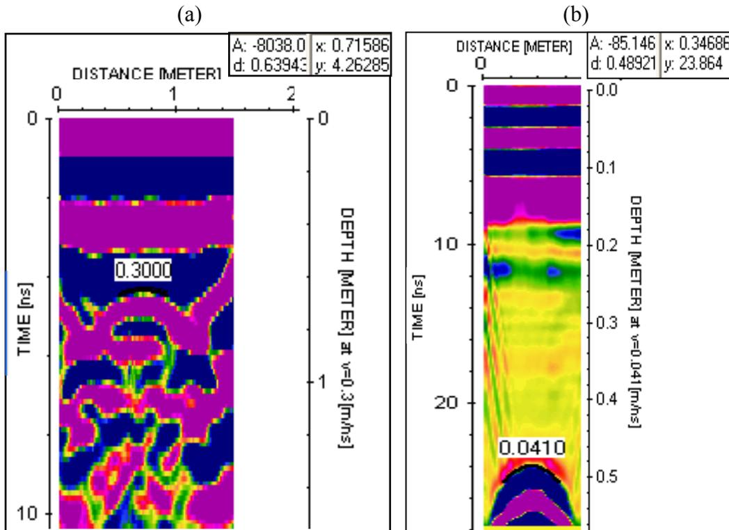
**Figure 6:** GPR profile obtained with 500 MHz antenna scanned over; (a) a cylindrical iron pipe with an atmosphere medium, (b) a cylindrical iron pipe with water medium. Objects are recognized by hyperbolic-shaped reflections.
