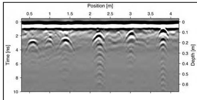
**Figure 2:** GPR profile obtained with a 1.5 GHz system scanned over six objects buried in sandy soil. The signal amplitude is plotted as a function of time (or depth) and position. Objects are recognized by hyperbolic-shaped reflections. Reflections from the ground surface appear as stripes at the top of the profile.
