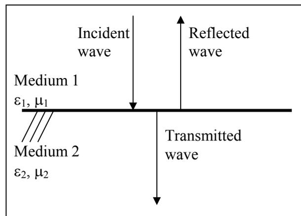
**Figure 3:** Reflection and transmission of a normal incident EM wave to a planar interface between two media.
