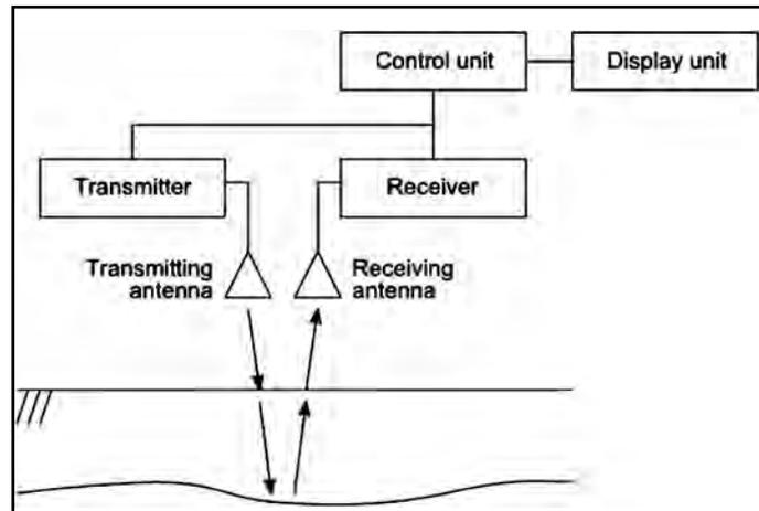
**Figure 1:** Schematic diagram of GPR system.
