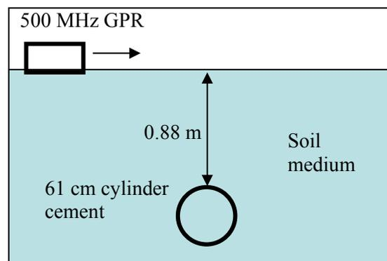
**Figure 5:** GPR study with 500 MHz antenna for cylinder cement drainage buried in soil medium.
