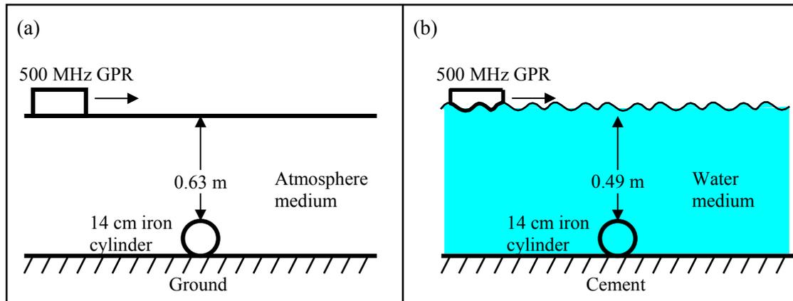
**Figure 4:** GPR study with 500 MHz antenna for cylinder iron pipe using different medium. (a) Atmosphere (b) Water.
