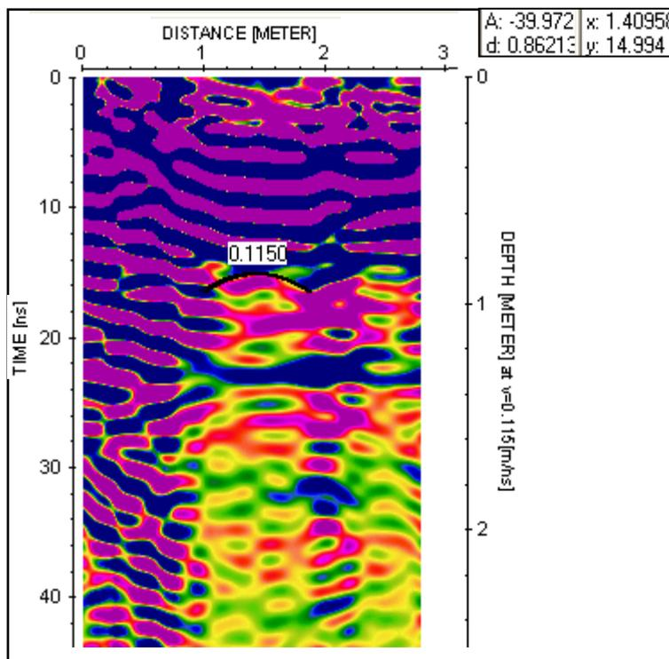
**Figure 7:** GPR profile obtained with 500 MHz antenna scanned over cylindrical cement drainage. Objects are recognized by hyperbolic-shaped reflections.
