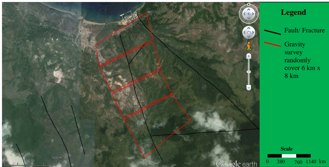
Figure 3: The gravity survey at Krueng Raya, Banda Aceh (Indonesia).
