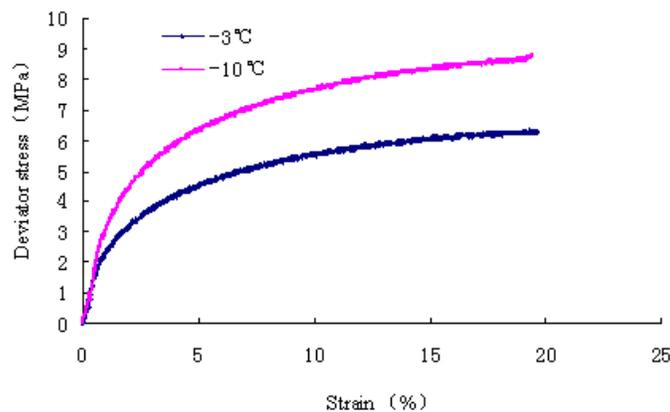
**Figure 4:** Stress–strain curves under different temperatures
