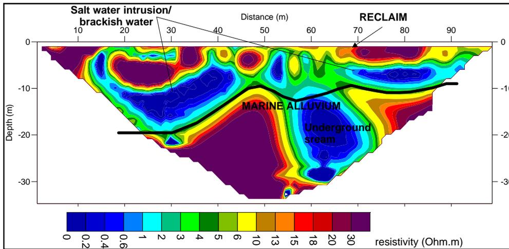
Figure 11: The 2-D resistivity inversion model of line L8.
