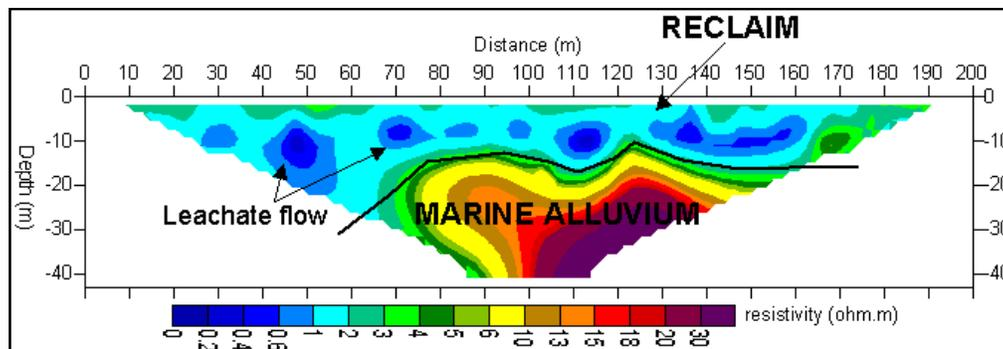
**Figure 4:** The 2-D resistivity inversion model of line L1
