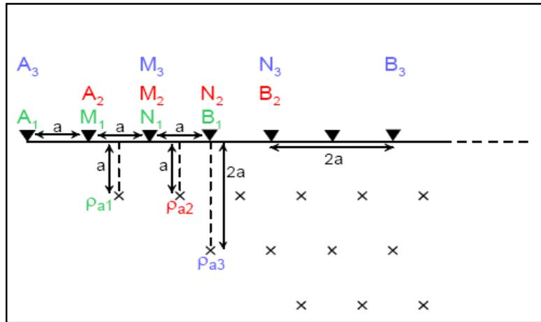
**Figure 2:** Conventional representation of the measured apparent resistivity  $\rho_a$  according to the electrode spacing ( $a$ ) between the electrodes (A, B, M and N).
