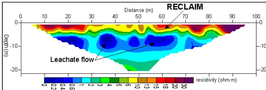
Figure 7: The 2-D resistivity inversion model of line L4
