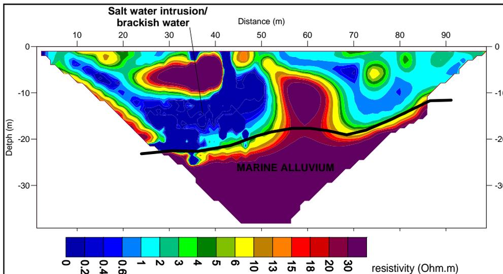
Figure 13: The 2-D resistivity inversion model of line L10.
