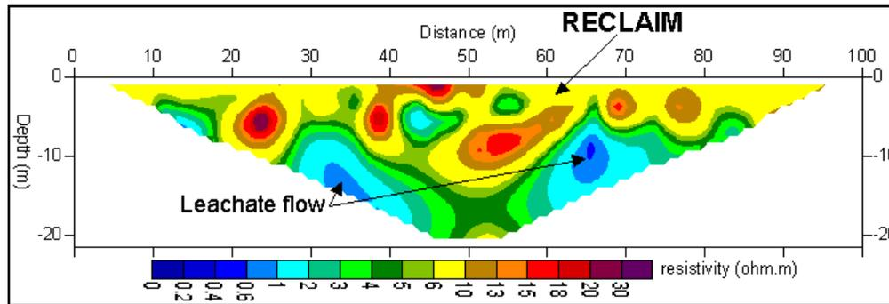
Figure 8: The 2-D resistivity inversion model of line L5
