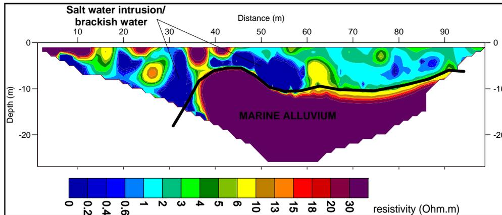
**Figure 14:** The 2-D resistivity inversion model of line L11.
