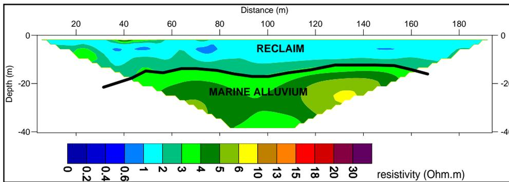
Figure 12: The 2-D resistivity inversion model of line L9.
