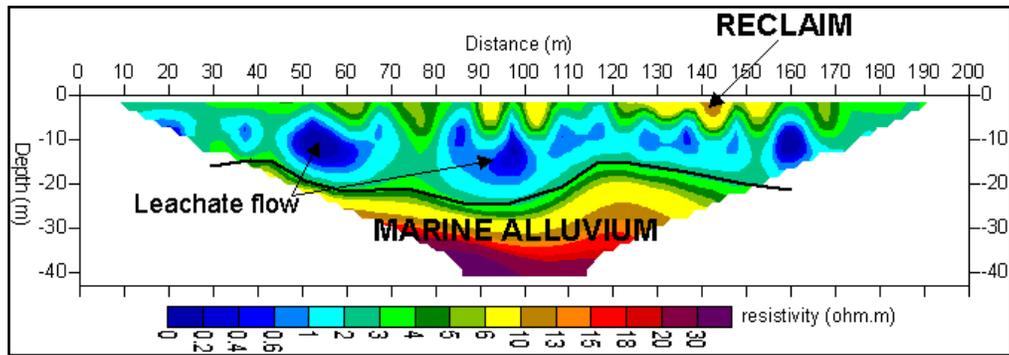
Figure 5: The 2-D resistivity inversion model of line L2
