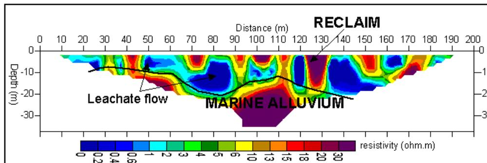
Figure 10: The 2-D resistivity inversion model of line L7
