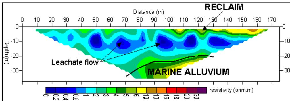
Figure 6: The 2-D resistivity inversion model of line L3
