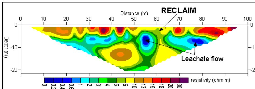
Figure 9: The 2-D resistivity inversion model of line L6
