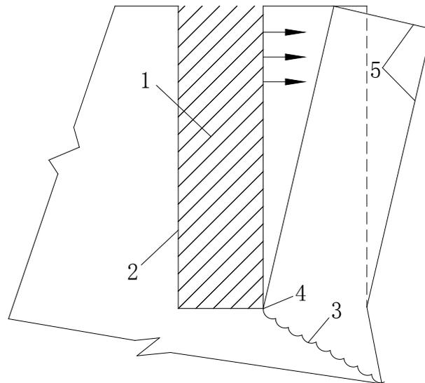
1. Static cracking agent; 2. Filling hole; 3. Micro crack; 4. Fracture stress; 5. Free surface
