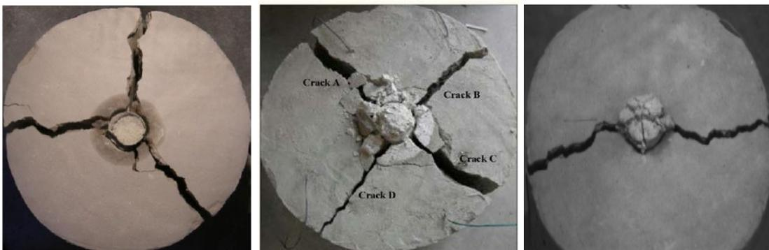
**Figure 14:** Single hole crack expansion in round broken material
