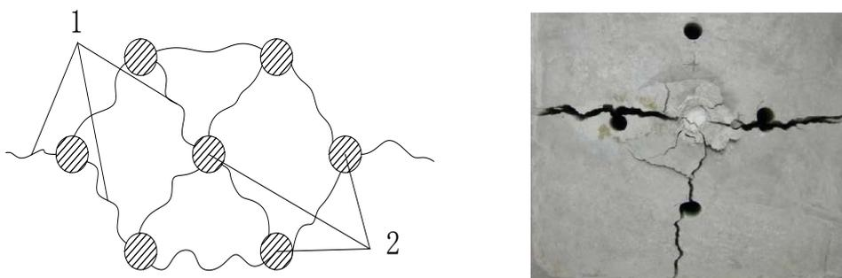
**Figure 17:** Schematic diagram of multi-hole crack expansion trend; Fig. 18 Actual situation of multi-hole crack development in lab (Du, 2008)
