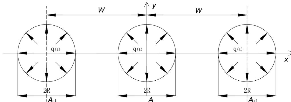
**Figure 6:** Single row multi-hole force model
