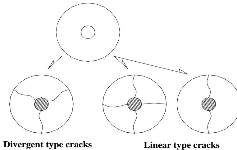
**Figure 13:** Schematic diagram of a single hole crack generation form (round broken material)
