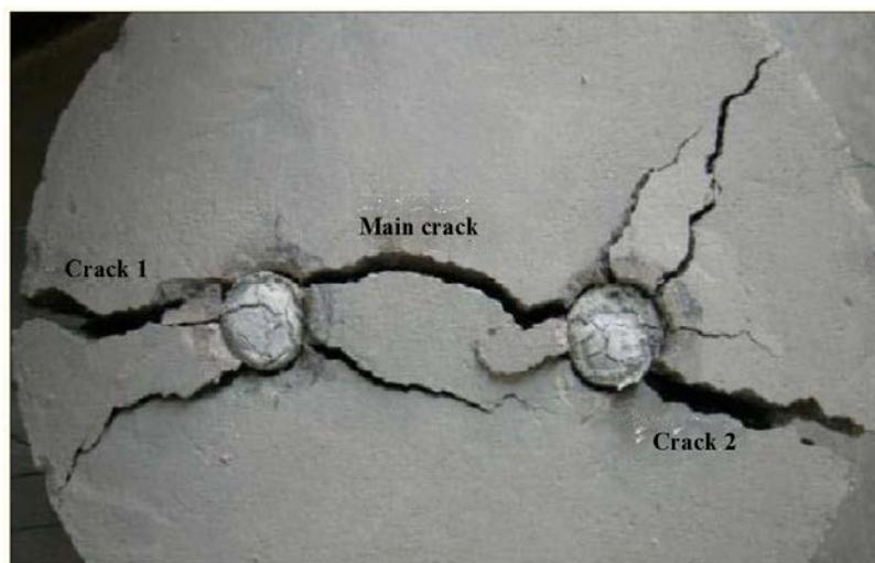
**Figure 16:** Actual situation of double hole crack development in lab (Du, 2008)
