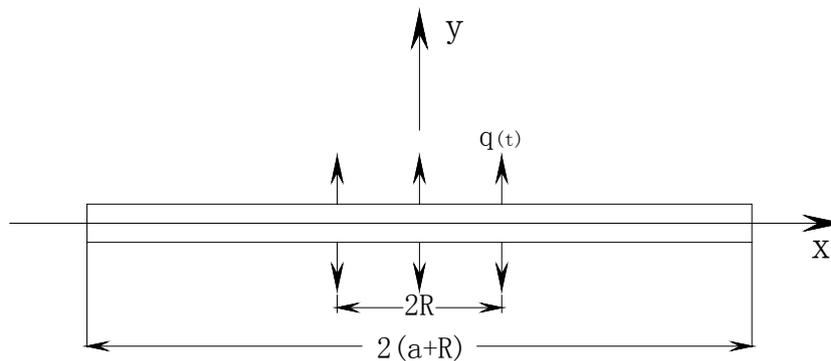
**Figure 8:** Uniform load acting on single hole fracture model
