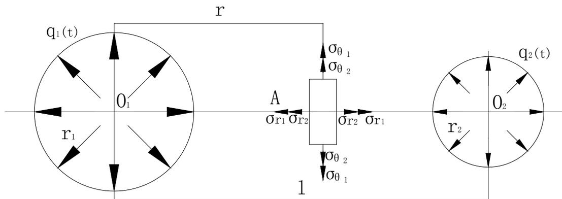
**Figure 5:** Force diagram of rock breaking model with two holes
