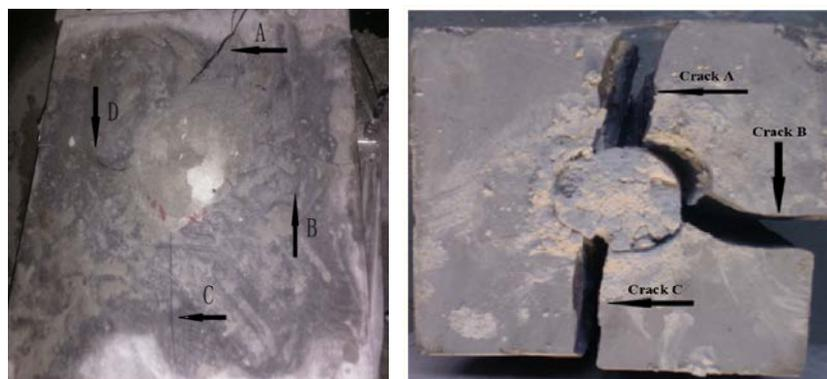
**Figure 12:** Single hole crack expansion in square broken material
