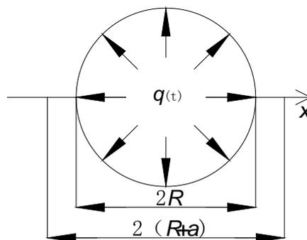
**Figure 7:** Single hole fracture model
