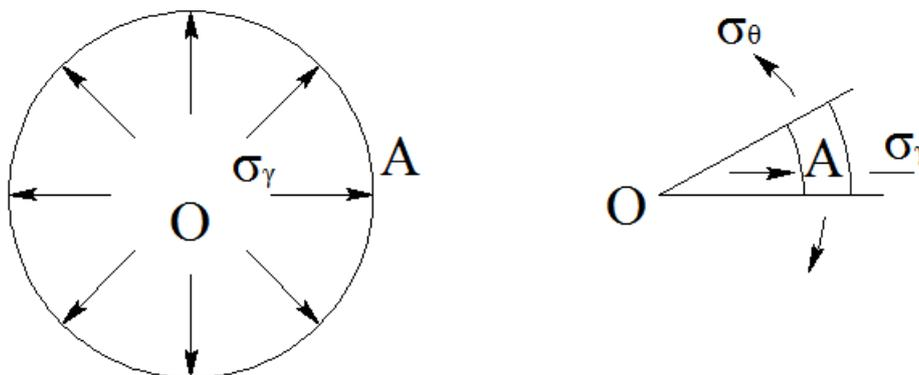
**Figure 1:** Radial and tangential stress state diagram of the hole unit body
