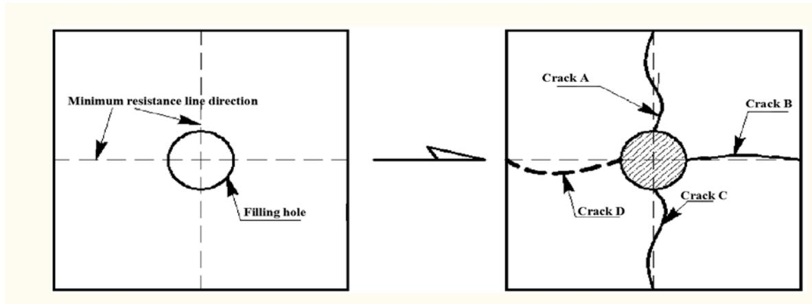
**Figure 11:** Schematic diagram of single hole crack generation form (square broken material)
