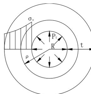
**Figure 3:** Schematic diagram of bounded single hole expansion stress variation
