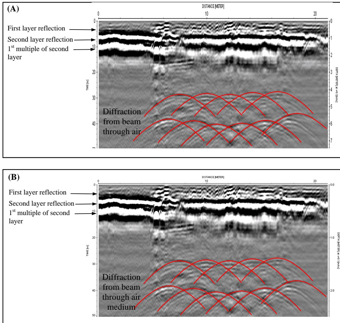
**Figure 5:** GPR results at Lamyong, Banda Aceh (Indonesia). (a) Processing with EM velocity of  $3 \times 10^8$  m/s, (b) Processing with EM velocity of  $1 \times 10^8$  m/s.
