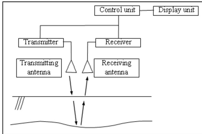
**Figure 1:** GPR system schematic diagram (Marwan, et al., 2014).
