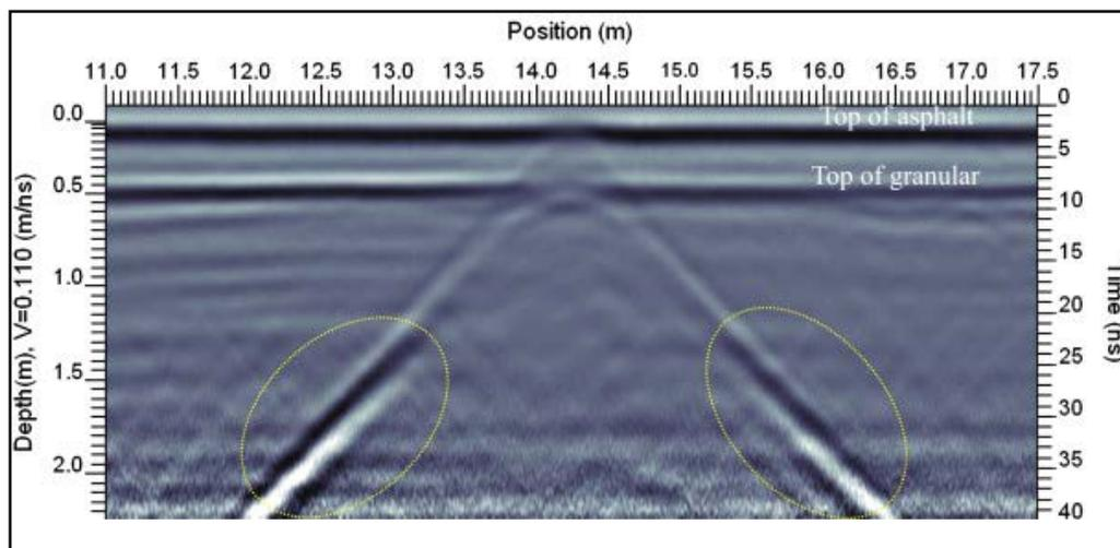
**Figure 2:** Cross-sections of 250 MHz GPR on asphalt pavement with thickness of 350 mm. The dashed circles indicate areas with shingling effects (Diamanti and Redman, 2012).
