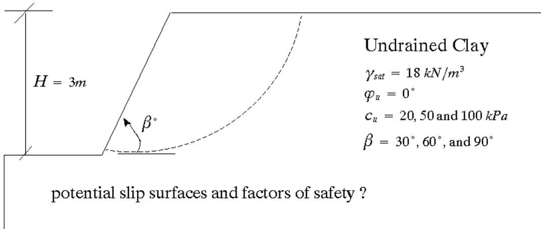
**Figure 1:** A traditional slope stability assignment
