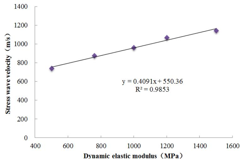
**Figure 8:** Relationship between dynamic elastic modulus and velocity curve of stress wave
