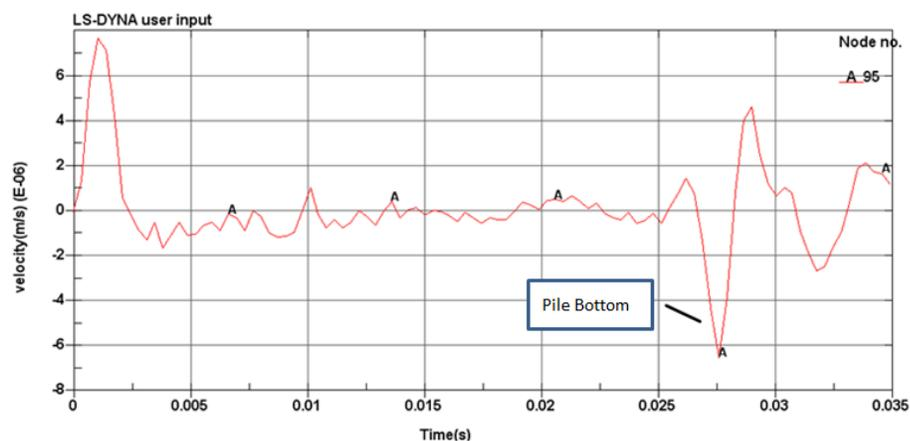
**Figure 2:** The simulation result of intact pile
