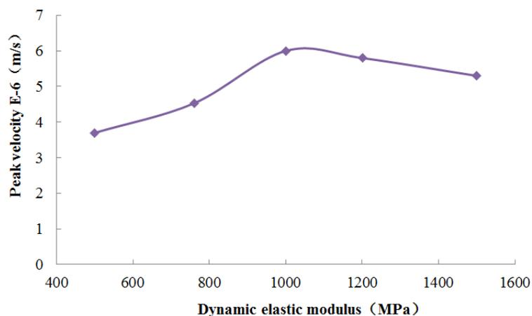
**Figure 9:** Relationship between speed peak at the bottom of the model and dynamic elastic modulus-
