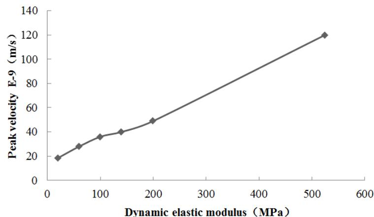
**Figure 5:** Relationship between speed peak at the bottom of the model and dynamic elastic modulus
