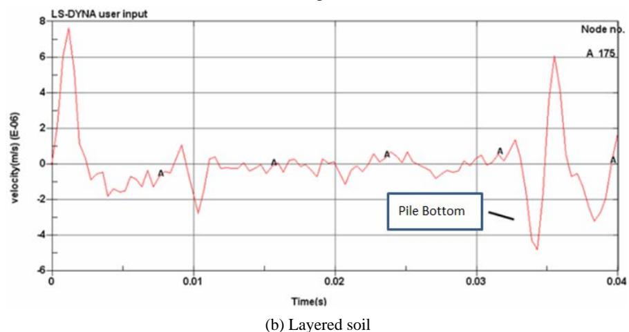
**Figure 6:** Waveform diagram for the soil around the pile is layer
