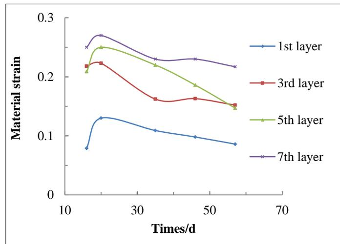
**Figure 5:** The variation of reinforced materials strain of geo-grid wrapping wall face versus the time
