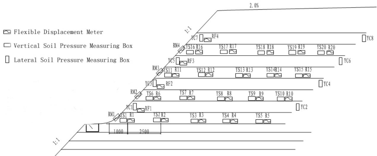
**Figure 1:** The arrangement plan of embankment monitoring test components
