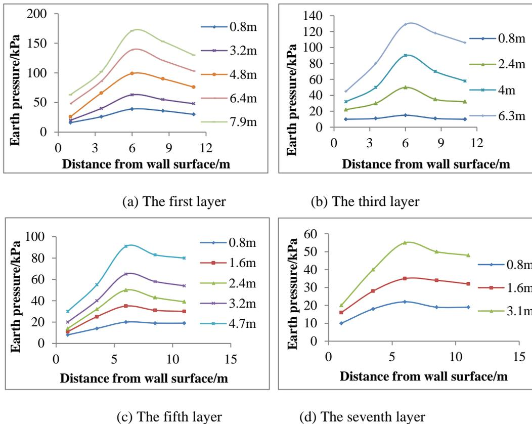
**Figure 2:** The variation of vertical soil pressure at different position (annotation: all graphic legend represents depth of filling above the first layer, the third layer, the fifth layer and the seventh layer)
