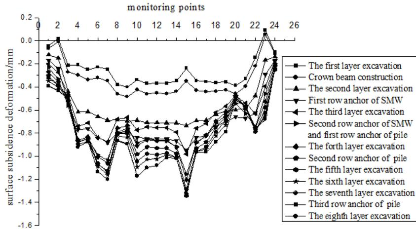
**Figure 7:** Surface settlement deformation near SMW
