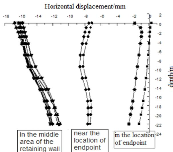
**Figure 10:** Horizontal displacement of double row pile retaining wall
