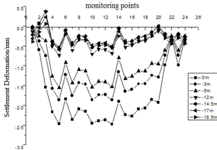
**Figure 12:** Settlement changes of double row pile surrounding soil
