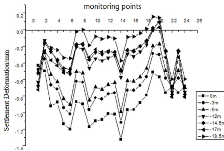
**Figure 13:** Settlement changes of soil around SMW retaining wall
