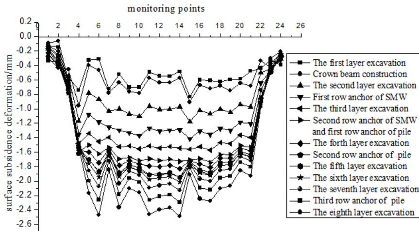
**Figure 8:** Surface settlement deformation near double row pile
