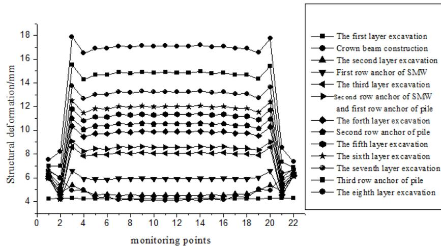
**Figure 6:** Deformation of double row piles supporting structure
