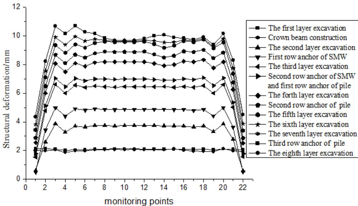
**Figure 5:** Supporting structure of SMW retaining wall deformation
