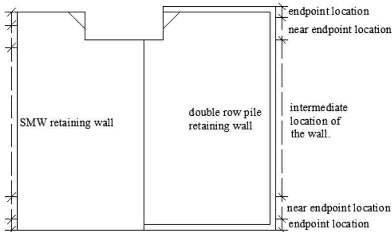
**Figure 9:** Different zones of a retaining wall
