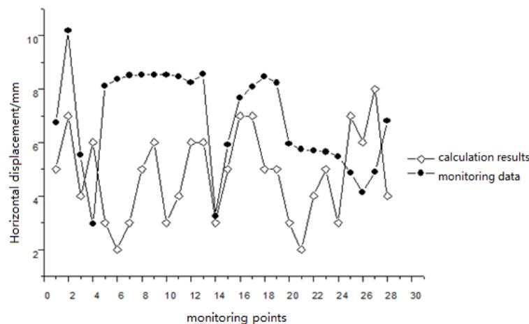
**Figure 4:** Analysis of horizontal displacement of pile top contrast
