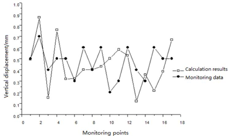
**Figure 5:** Analysis of vertical displacement of pile top contrast
