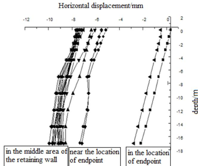
**Figure 11:** Horizontal displacement of SMW retaining wall
