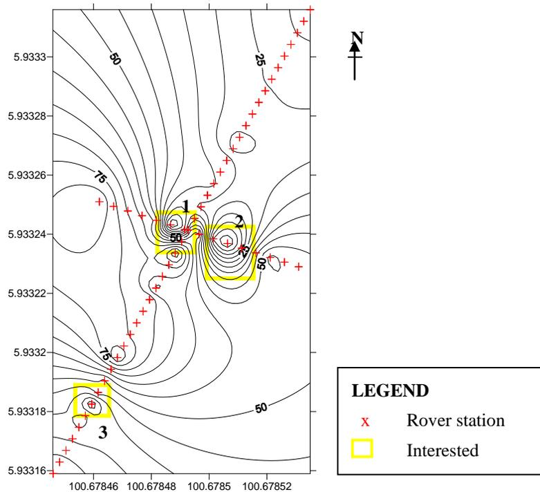
**Figure 4:** Magnetic anomaly contour map of study area with rover stations.
