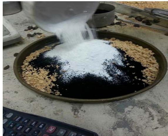
**Figure 2:** Sample of clay soil, rubber powder and lime
