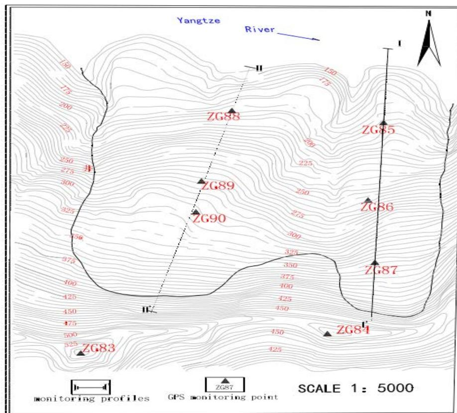
**Figure 2:** Topographical map of Shuping landslide, with location of GPS monitoring points
