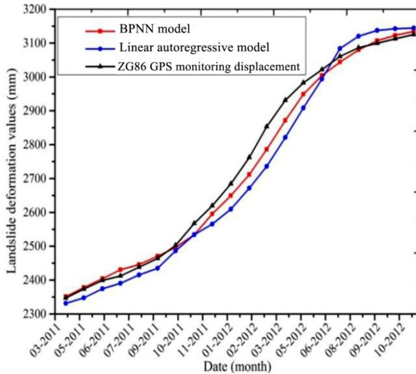
**Figure 5:** Comparison of predicted and measured monthly cumulative displacement values
