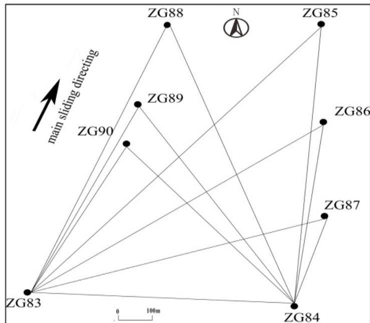
**Figure 3:** GPS monitoring network
