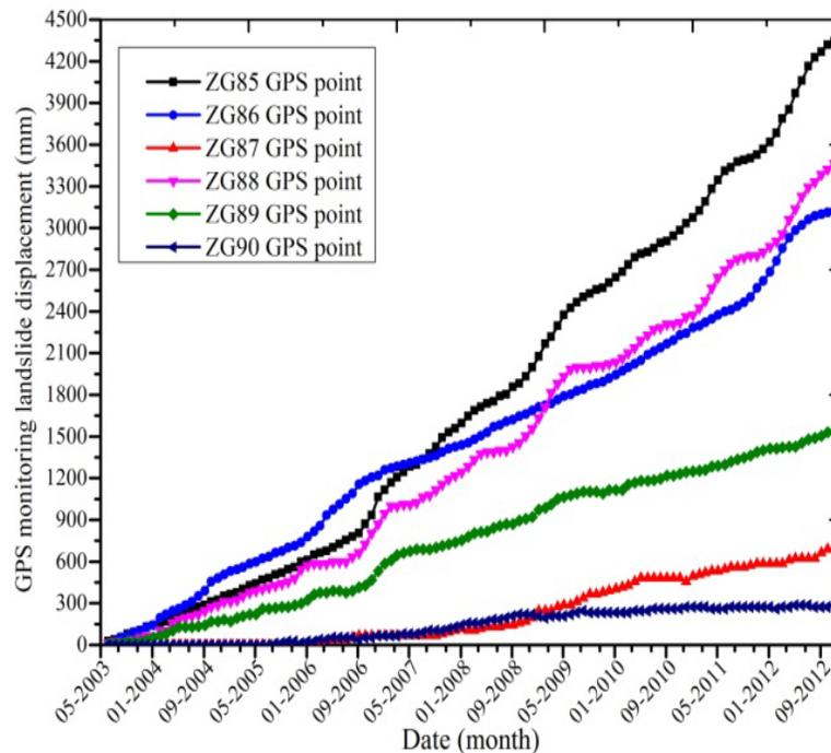
**Figure 4:** Monthly Cumulative displacement time series monitored by GPS
