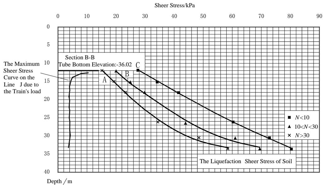
**Figure 6:** Maximum shear stress and foundation liquefaction shear stress on line J due to train vibration
