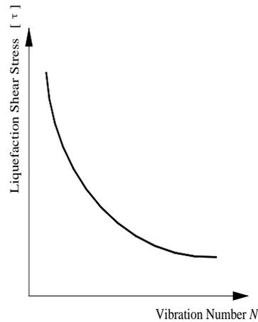
**Figure 3:** Relationship between liquefaction shear stress ratio and liquefaction vibrating number
