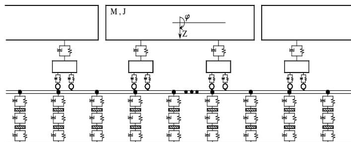
**Figure 4:** Vehicle/Track coupling dynamic model
