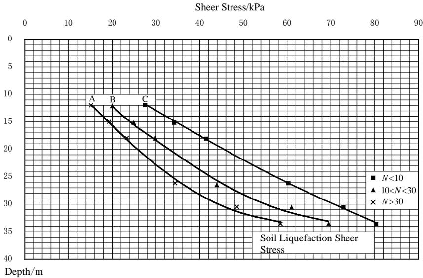
**Figure 2:** Foundation liquefaction shear stress
