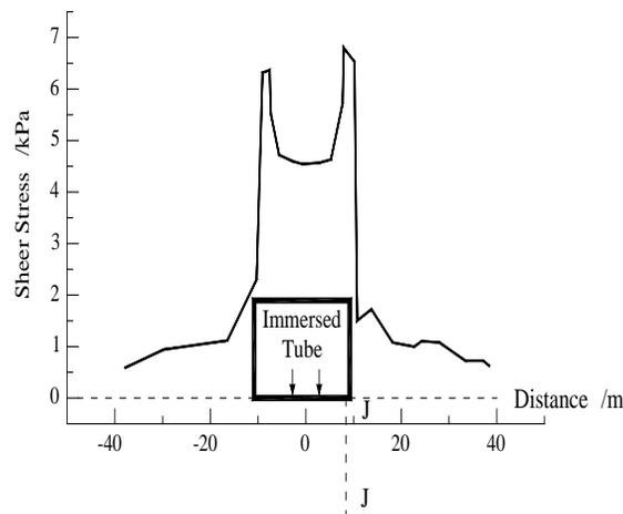
**Figure 5:** Horizontal distribution of maximum sheer stress at elevation of immersed tube bottom
