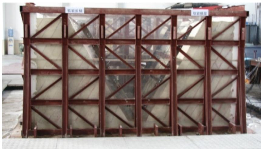
**Figure 2: Slope model placed on the shaking table**
