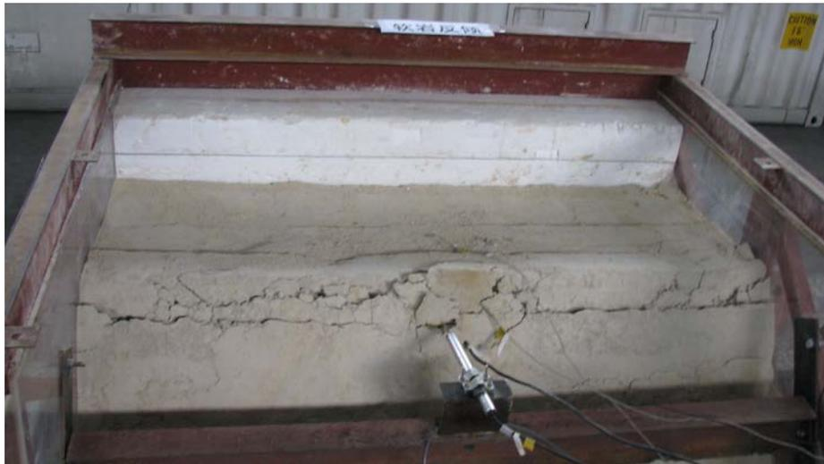
**Figure 10:** bending and caving in slope shoulder
