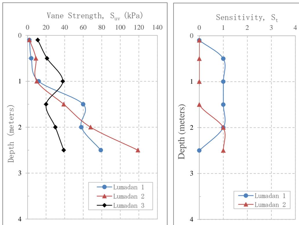
**Figure 3:** Vane Shear Test Result for Lumadan Peat.
