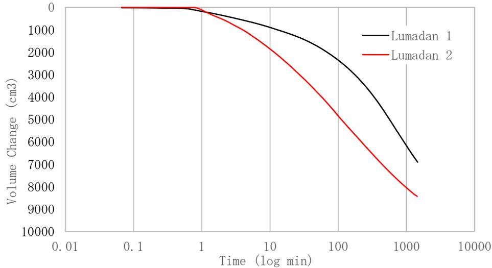
**Figure 4:** Volume change versus square root of time for a Lumadan Peat specimen under effective stress,  $\sigma = 100$  kPa.
