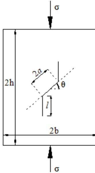
**Figure 2:** A unit cell model for a sliding crack under uniaxial compression
