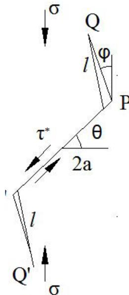
**Figure 1:** The sliding model for a microcrack
