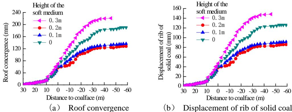
**Figure 7:** Deformation curves with different height of the soft medium
