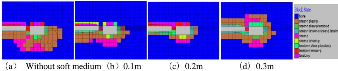
Figure 4: Plastic zone of roadway surrounding rock in different height of the soft medium
