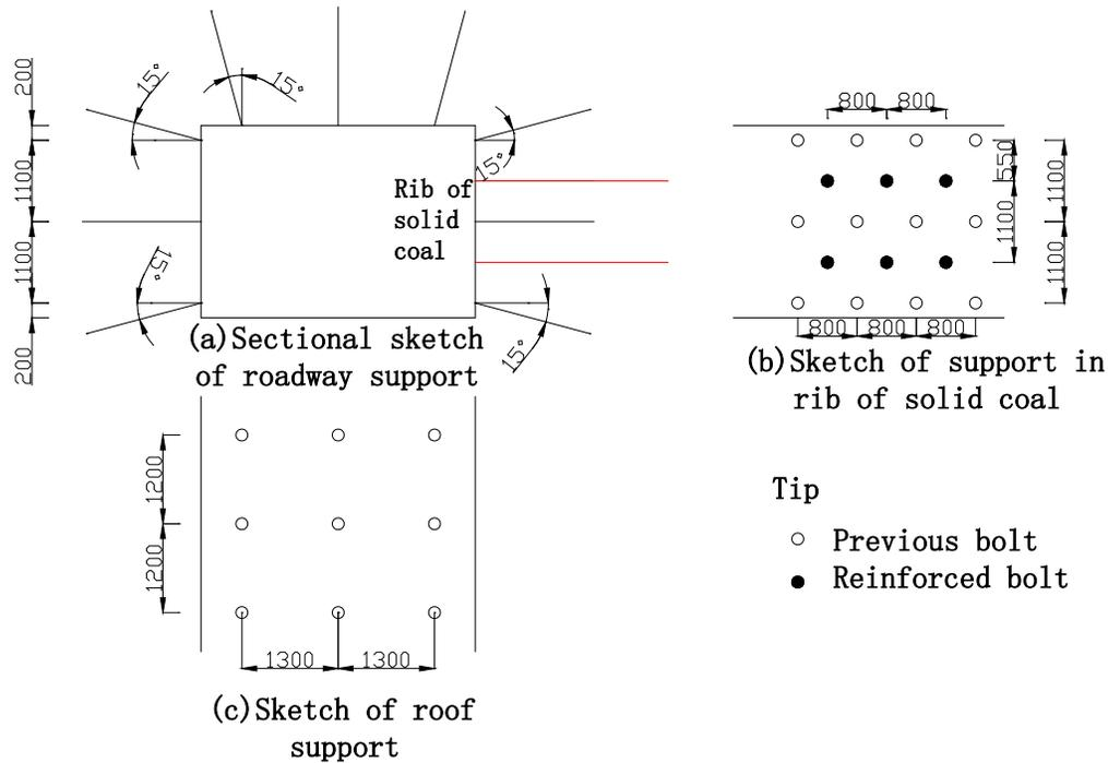
**Figure 1:** Bolting support sketch after reinforcement (unit: mm)
