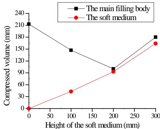
Figure 6: The relationship between compressed volume and height of the soft medium
