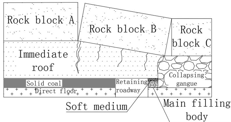
**Figure 2:** Structure diagram of the soft medium connecting the roof
