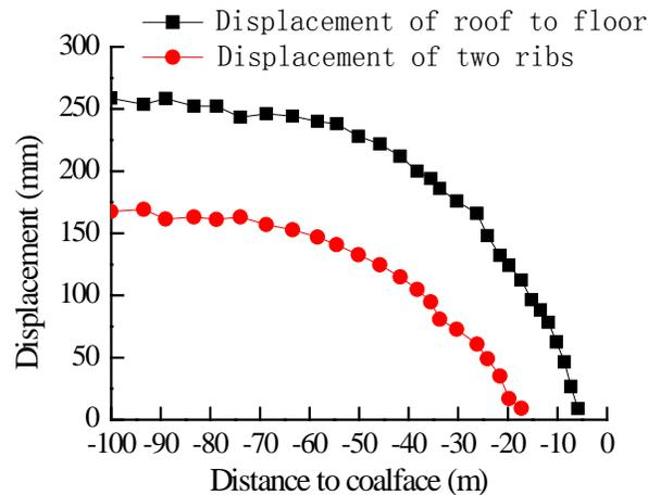
**Figure 8:** Relationship between displacement of surrounding rock and distance of working face
