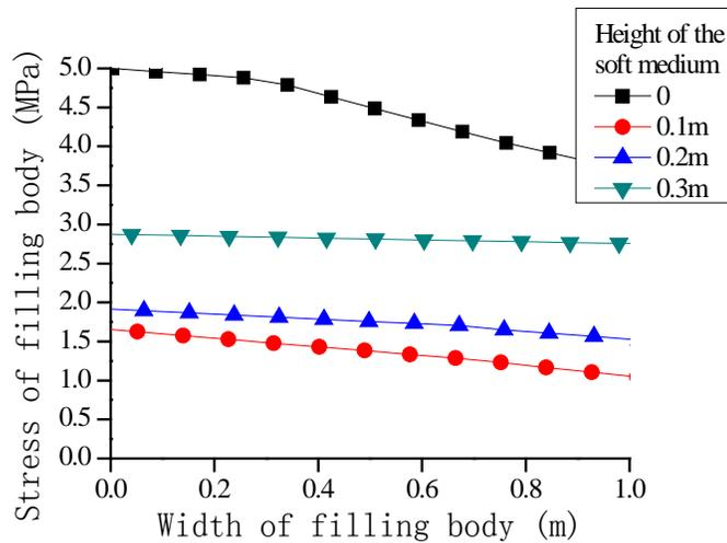
Figure 5: Backfill stress with different height of the soft medium
