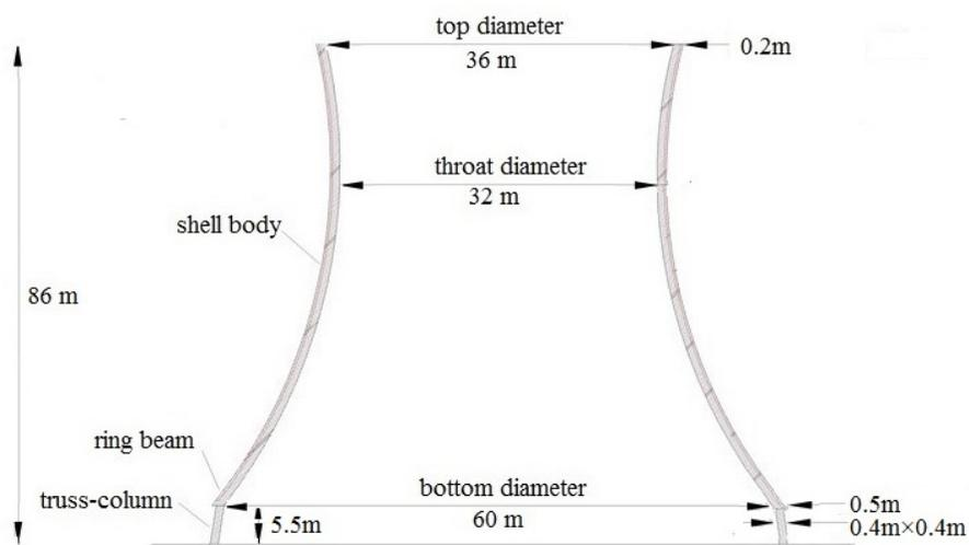
**Figure 2:** Profile of the cooling tower
