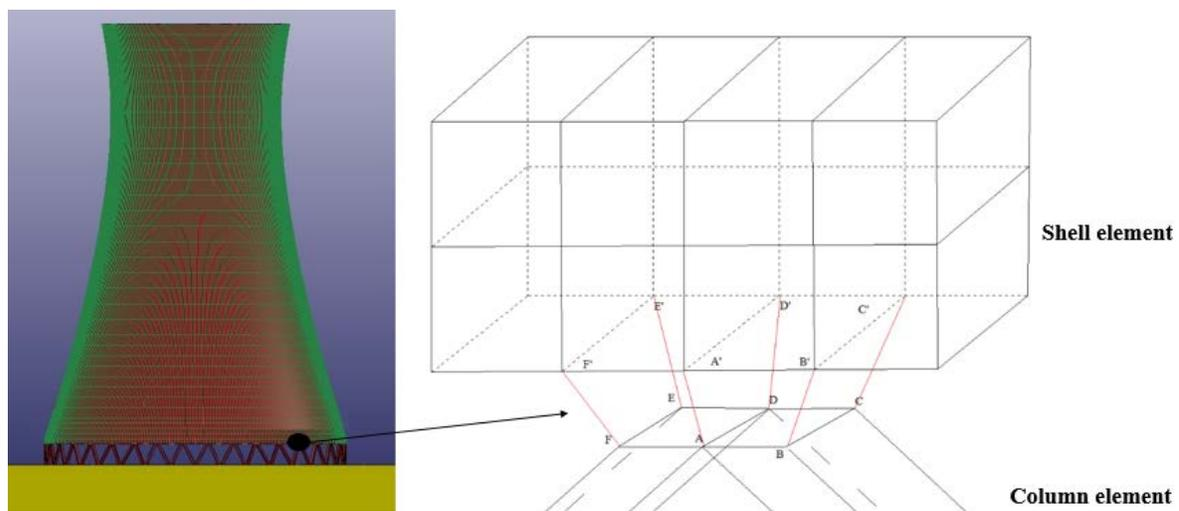
**Figure 4:** Connection of shell elements with column elements.
