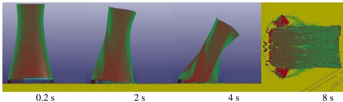
**Figure 6:** Simulated collapsed process of the cooling tower
