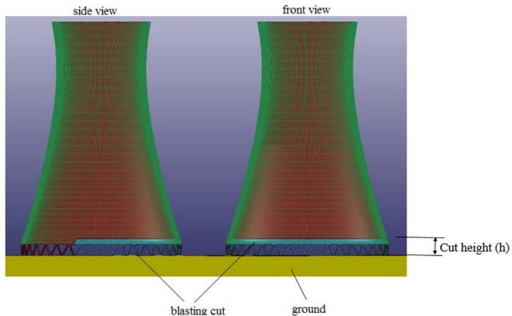
**Figure 5:** The model of the cooling water with blasting cut
