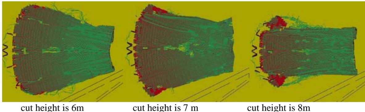
**Figure 7:** The tower collapsed range under different cut height
