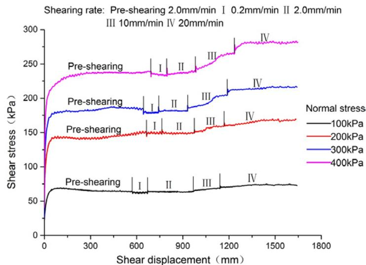
**Figure 5:** Relationships between shear stress and shear displacement
