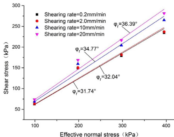
**Figure 6:** Relationships between shear strength and effective normal stress
