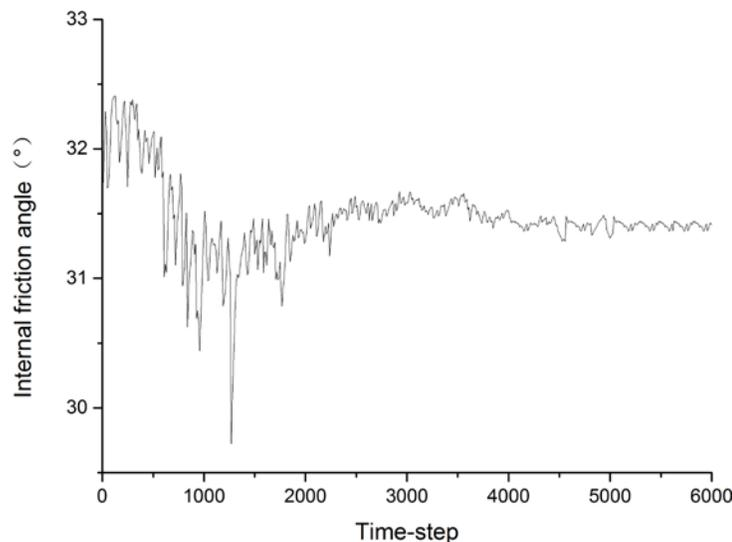
**Figure 10:** Relationship between internal friction angle and time-step
