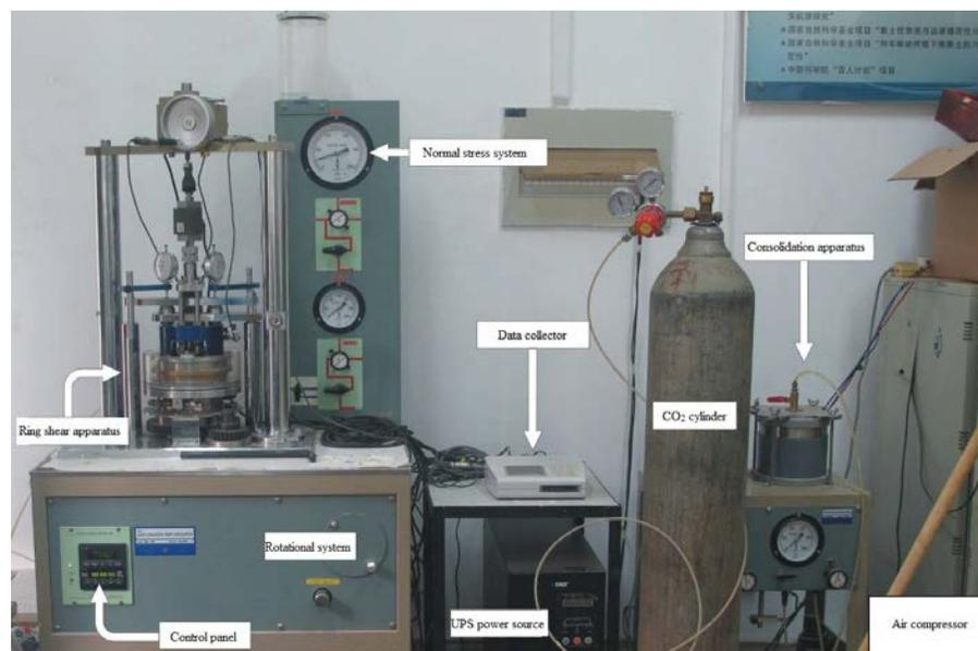
**Figure 4:** System of DTA-138 ring shear apparatus
