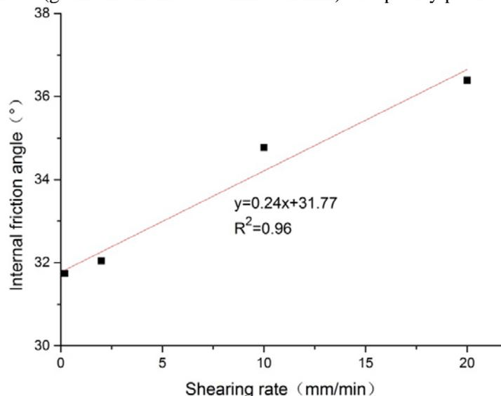
**Figure 7:** Relationship between internal friction angle and shearing rate
