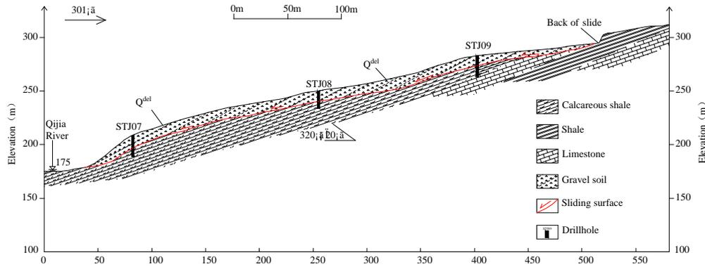
**Figure 1:** Longitudinal section of Sanjiaotan landslide(unit: m)
