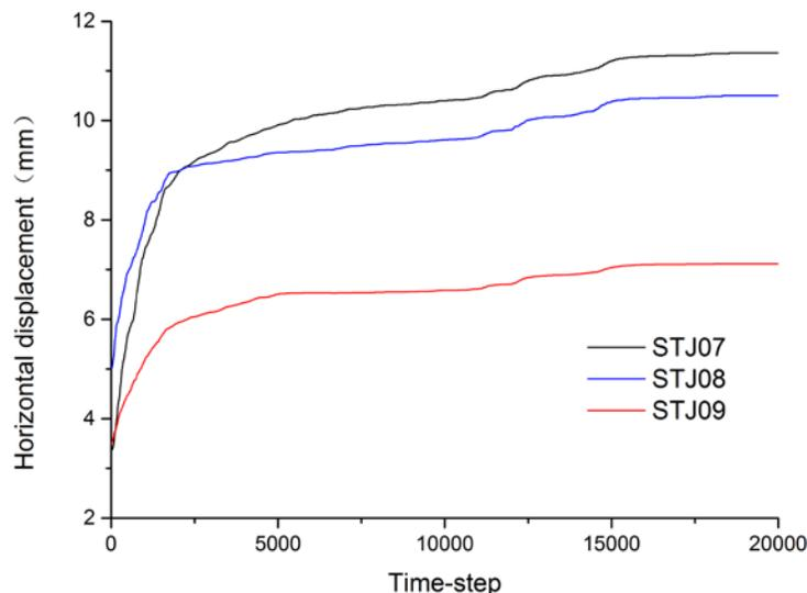
**Figure 9:** Relationships between horizontal displacement of monitoring sites and time-step
