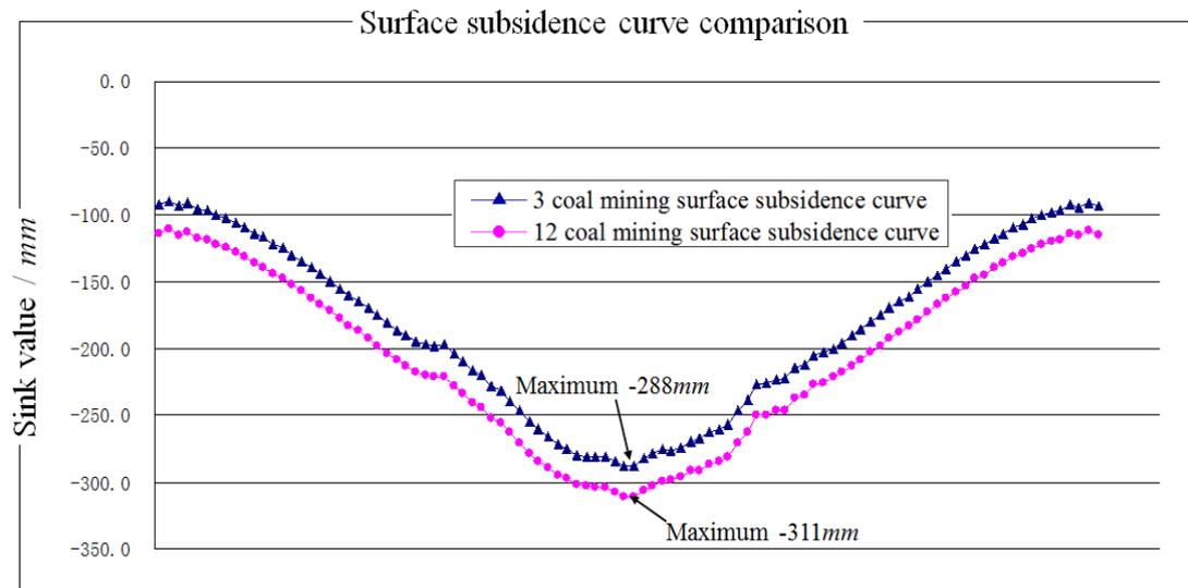
**Figure 7:** The surface subsidence curve contrast diagram
