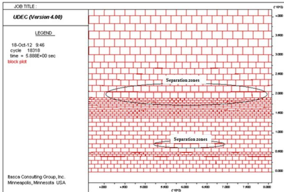
**Figure 4:** Deformation and failure of 3<sub>up</sub># Coal (completely mining) and 12# Coal (strip mining)
