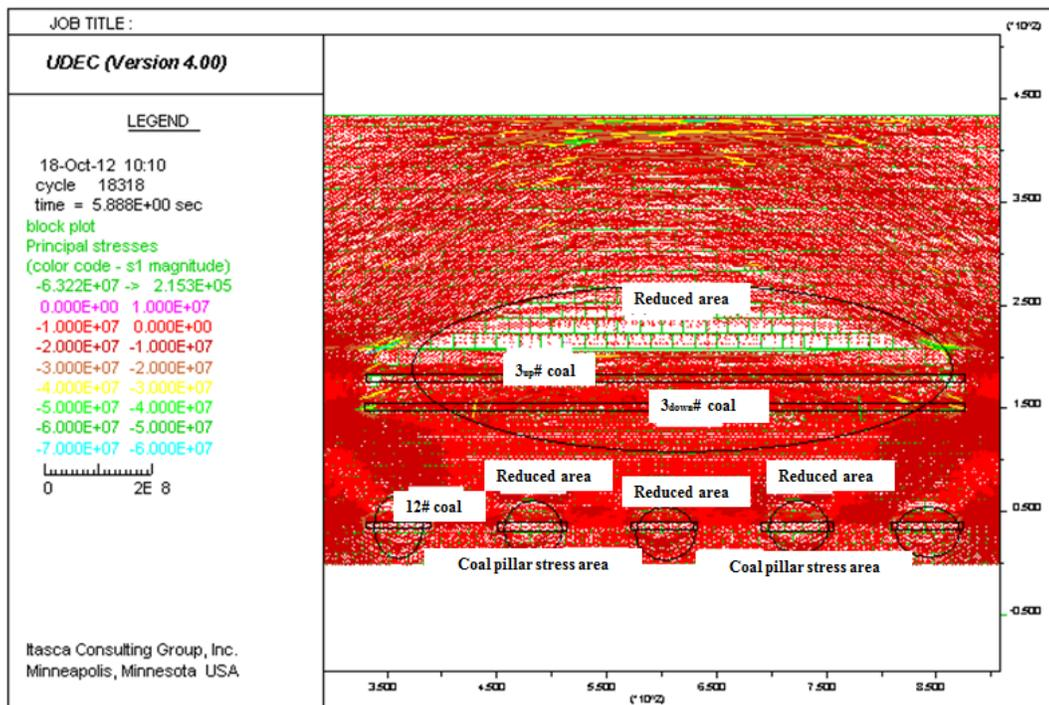
**Figure 3:** Stress arch evolution of 3<sub>up</sub># Coal (completely mining) and 12# Coal (strip mining)
