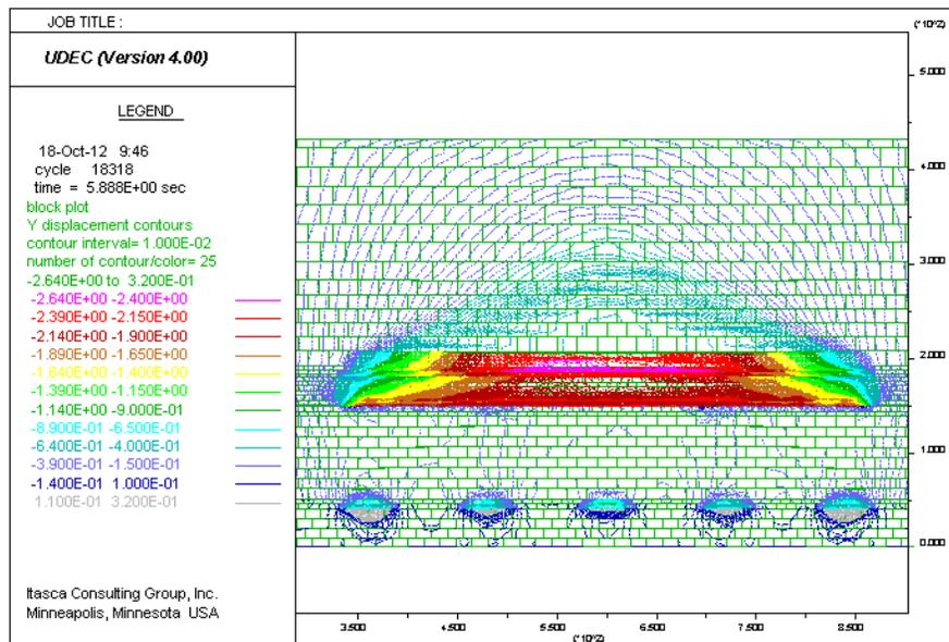
**Figure 6:** Displacement isoline of 3<sub>up</sub># Coal (completely mining) and 12# Coal (strip mining)
