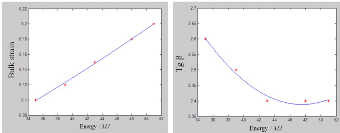
**Figure 8:** Relationship between energy and body strain Fig 9 Relationship between energy and  $tg\beta$
