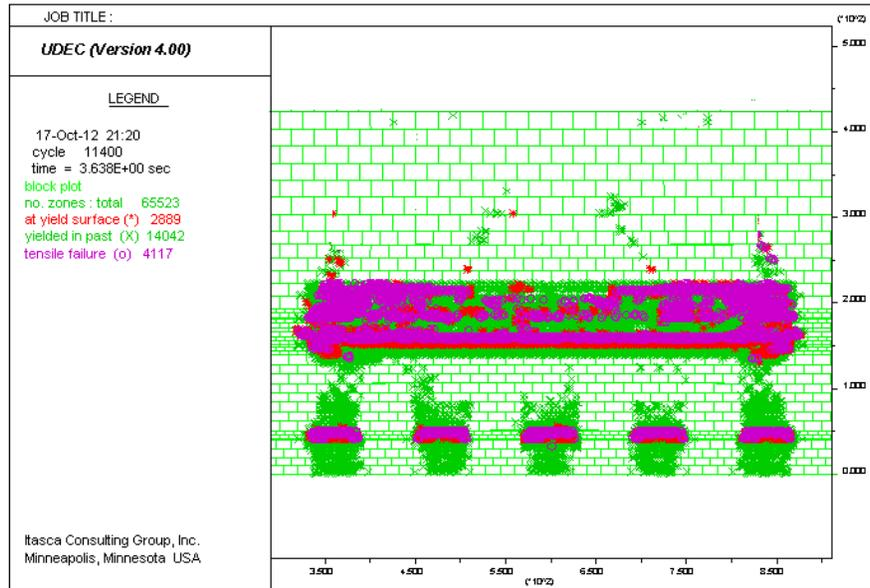
**Figure 5:** plastic zone distribution of 3<sub>up</sub># Coal (completely mining) and 12# Coal (strip mining)
