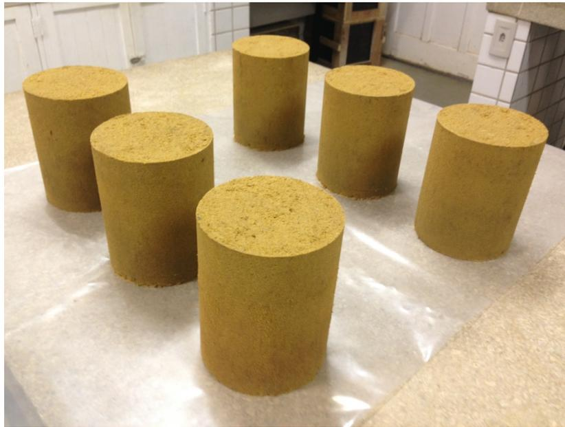
**Figure 2:** Cement-improved CDW specimens.
