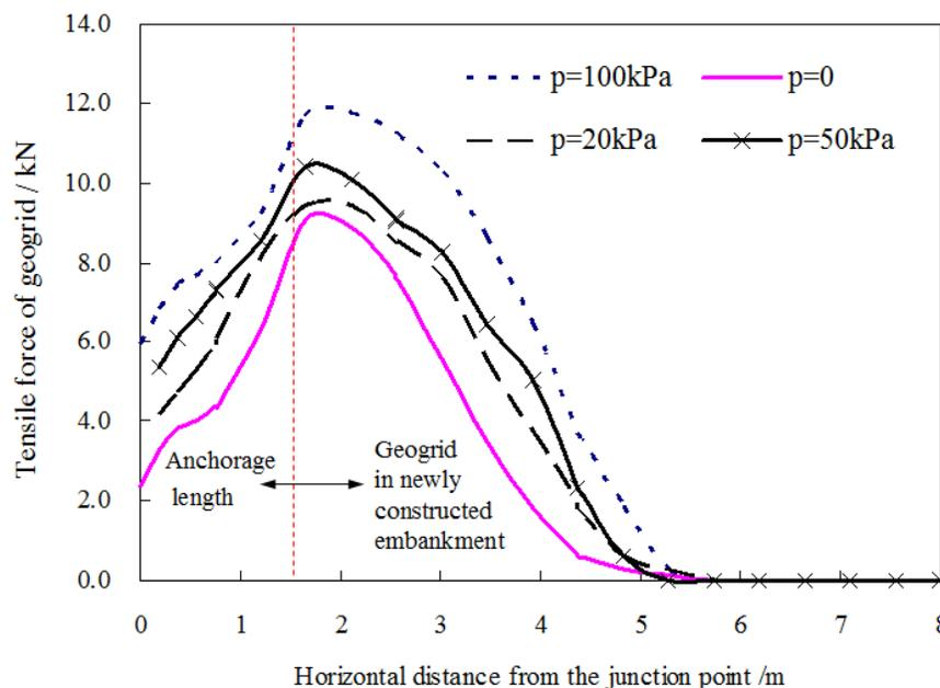
**Figure 5:** Tensile force of bottom geogrid
