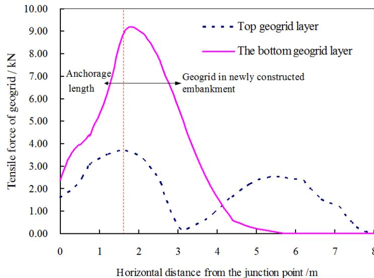
**Figure 4:** Tensile force of geogrid
