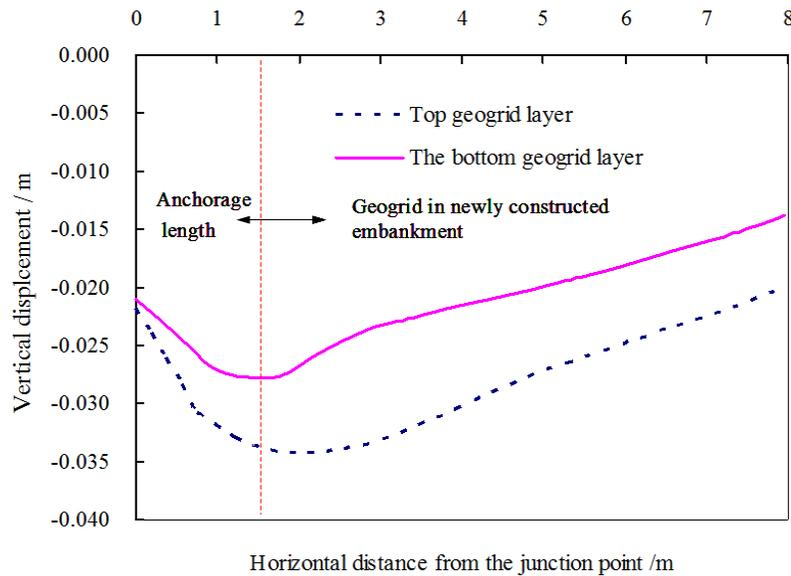
**Figure 3:** Vertical displacement of geogrid
