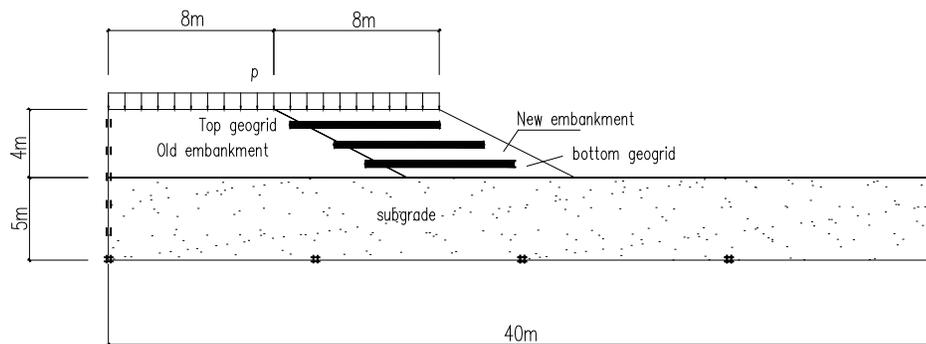
**Figure 1:** Geometry model for numerical simulation
