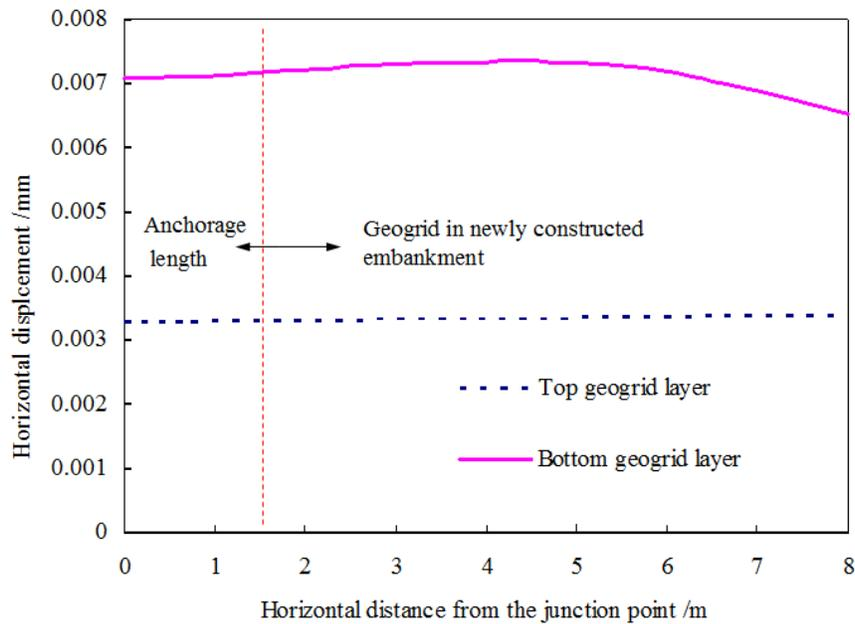
**Figure 2:** Horizontal displacements of geogrid
