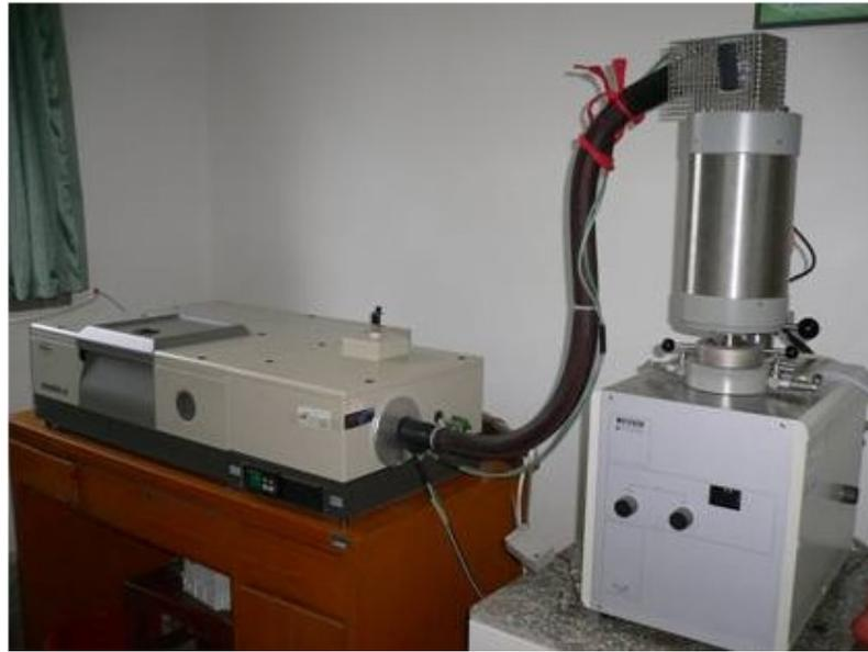
**Figure 2:** Thermal gravity combined with infrared spectrum instrument
