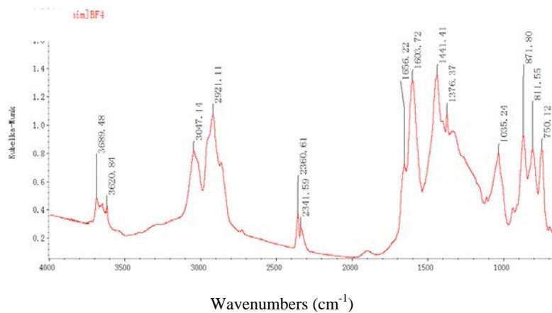
**Figure 6:** FTIR spectrum of the [HOEmim]BF<sub>4</sub> pretreated coal
