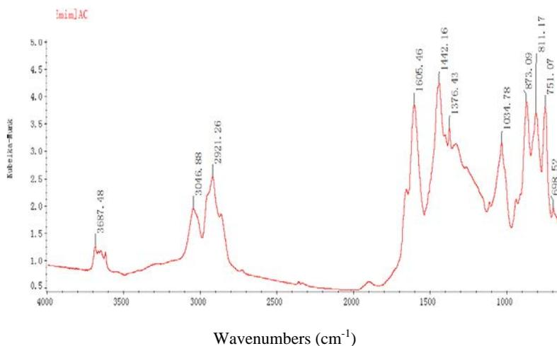
**Figure 4:** FTIR spectrum of the [Emim]AC pretreated coal
