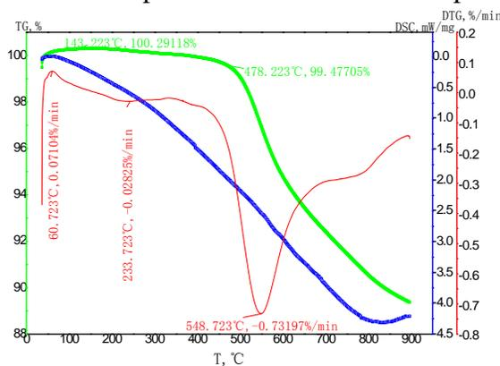
**Figure 11:** TG-DTG-DSC curves and inflection points of the [HOEmim]BF<sub>4</sub> pretreated coal
