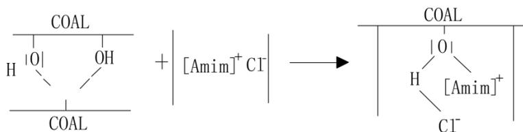
**Figure 7:** Interaction mechanism of coal and [Amim]Cl
