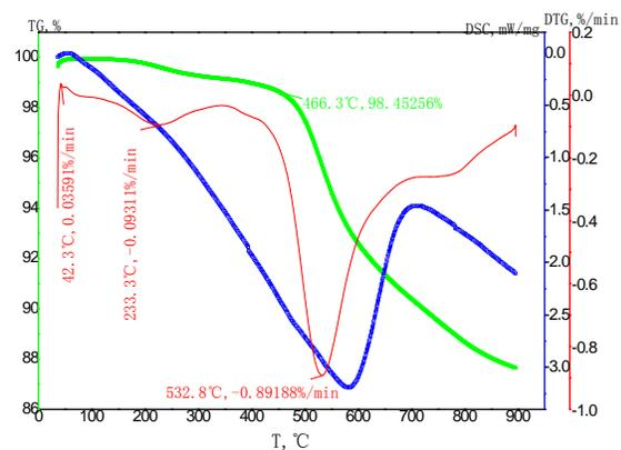
**Figure 10:** TG-DTG-DSC curves and inflection points of the [Amim]Cl pretreated coal
