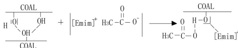
**Figure 6:** Interaction mechanism of coal and [Emim]AC
