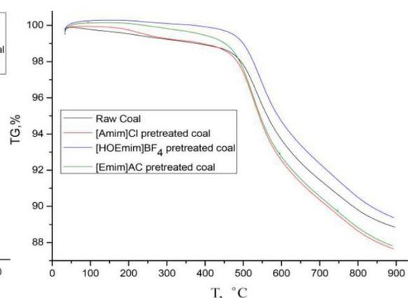
Figure 11: DTG curves of the raw coal and three ILs pretreated coals
