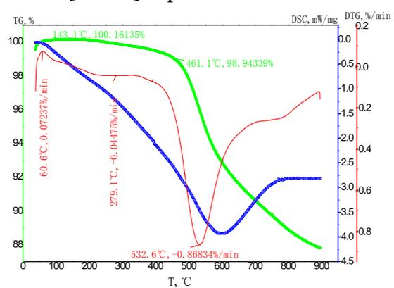
**Figure 12:** TG-DTG-DSC curves and inflection points of the [Emim]AC pretreated coal
