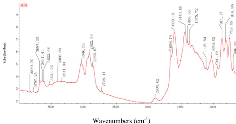
**Figure 3:** FTIR spectrum of the raw coal
