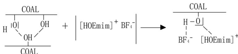
**Figure 8:** Interaction mechanism of coal and [HOEmim]BF<sub>4</sub>
