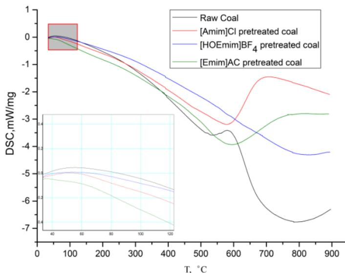
**Figure 12:** DSC curves of the raw coal and three ILs pretreated coals
