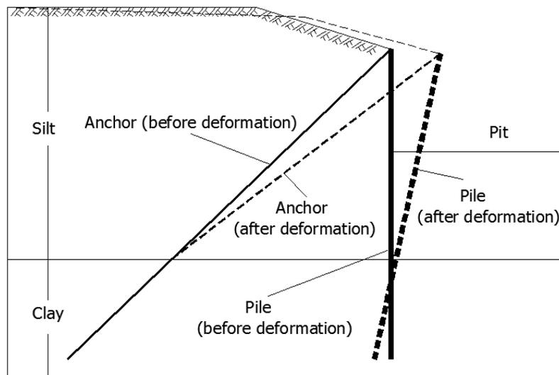
**Figure 4:** Schematic of rotation by pile anchor structure
