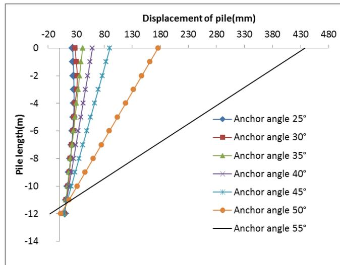
**Figure 9:** Horizontal displacement contrast of pile
