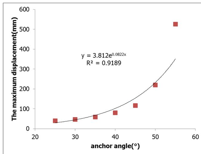
**Figure 13:** The maximum displacement of anchor
