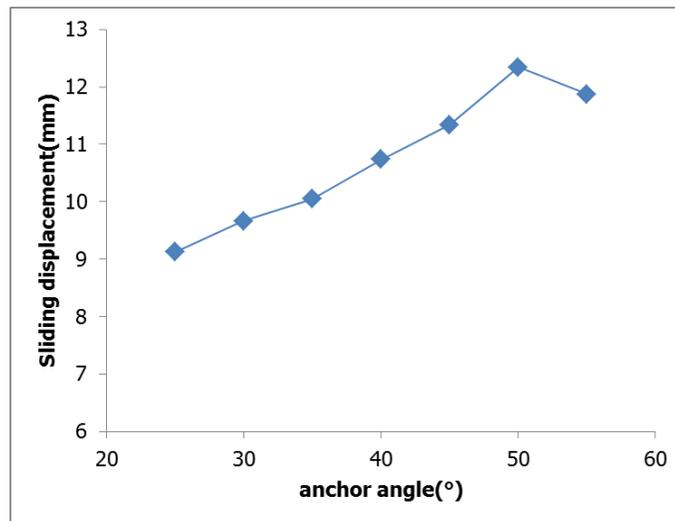
**Figure 14:** Sliding displacement of anchoring segment
