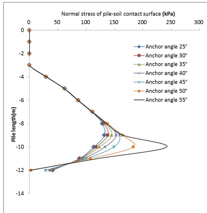
**Figure 18:** NS distribution of pile-soil contact surface
