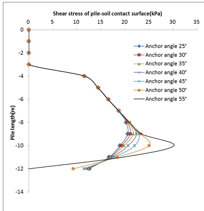
Figure 16: SS distribution of pile-soil interface (right side)
