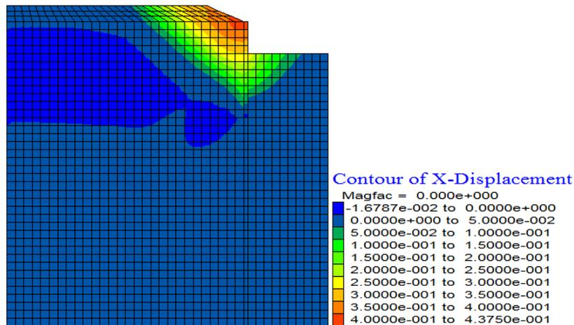
**Figure 6:** Deformation cloud of pit
