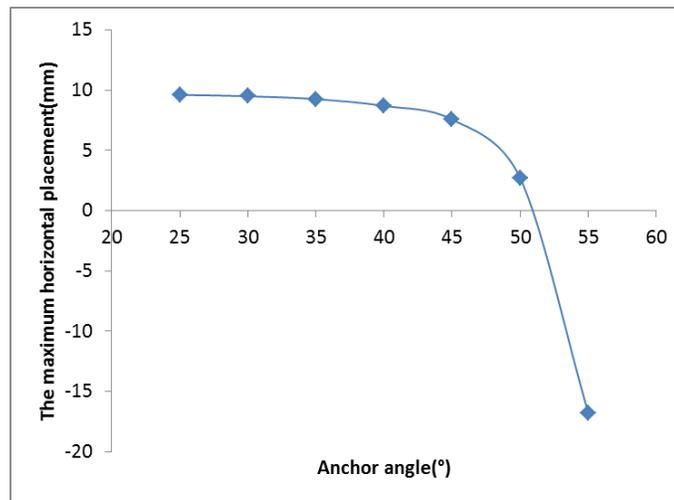
**Figure 10** Horizontal displacement contrast of pile bottom
