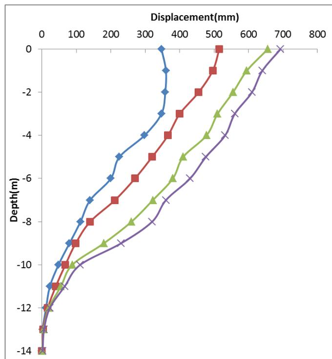
**Figure 3:** Monitoring data of horizontal displacement
