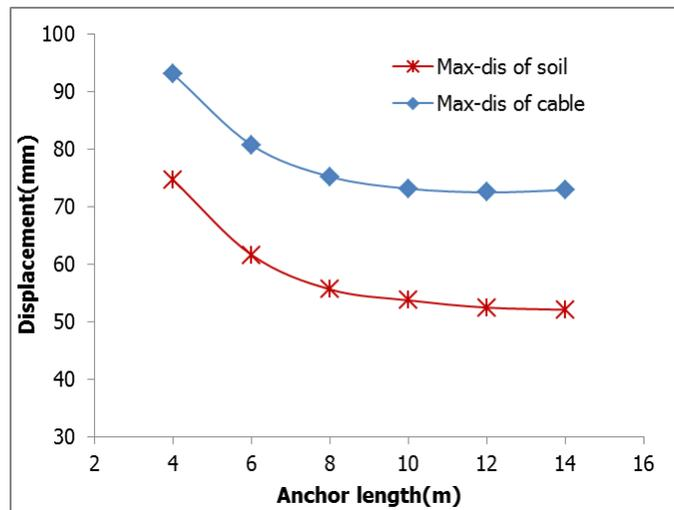
**Figure 19:** Relationship of anchor length and displacement
