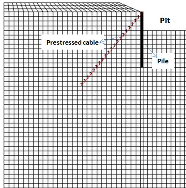
**Figure 5:** The element grid used in the numerical model
