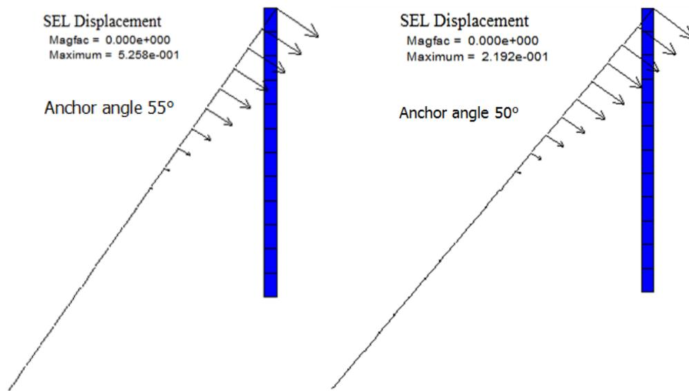
**Figure 12:** Vector of anchor deformation
