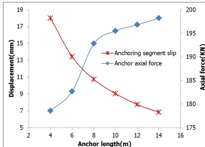
**Figure 20:** Relationship of anchor length and displacement
