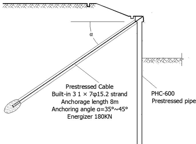
**Figure 1: Design schematic of pit cross-section**
