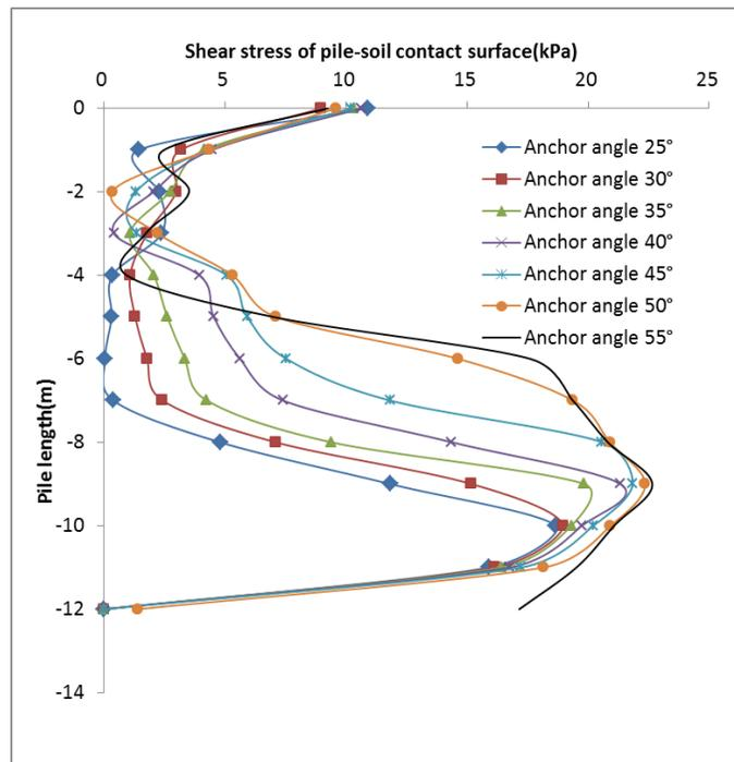
Figure 15: SS distribution of pile-soil interface (left side)
