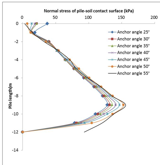
**Figure 17:** NS distribution of pile-soil contact surface
