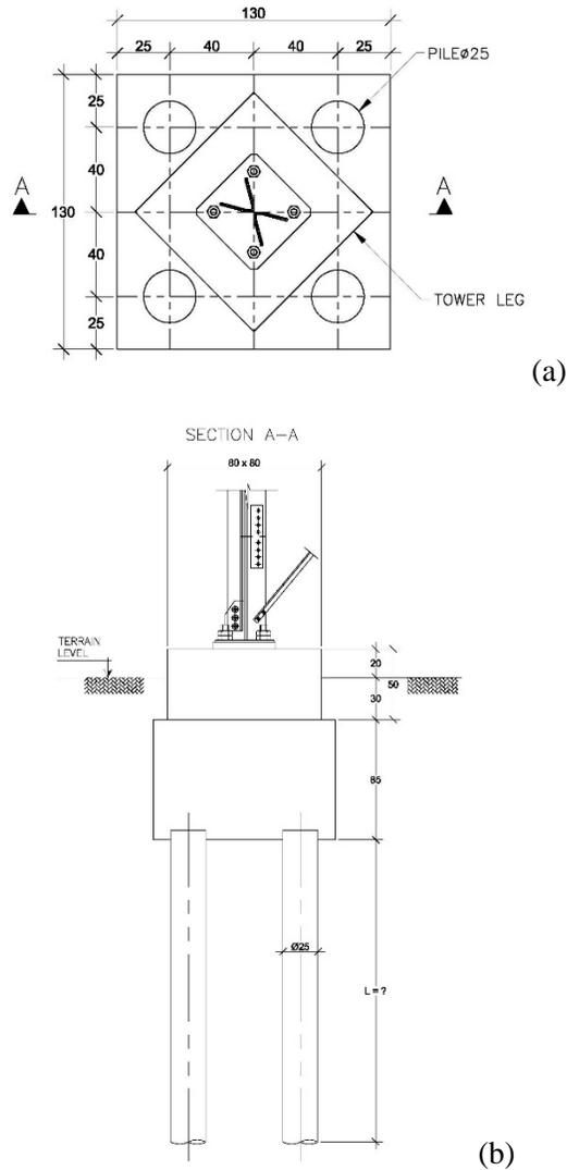
**Figure 4:** Foundation block detail: (a) plan view of a block, and (b) elevation of the block depicting two root-piles.
