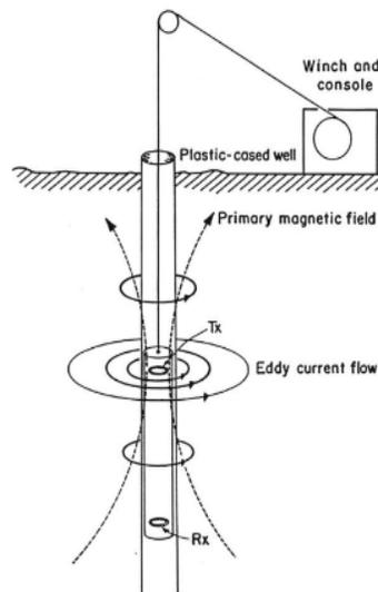
**Figure 1:** Illustration of the working principle of the Induction Logging Test (McNeill, 1990).
