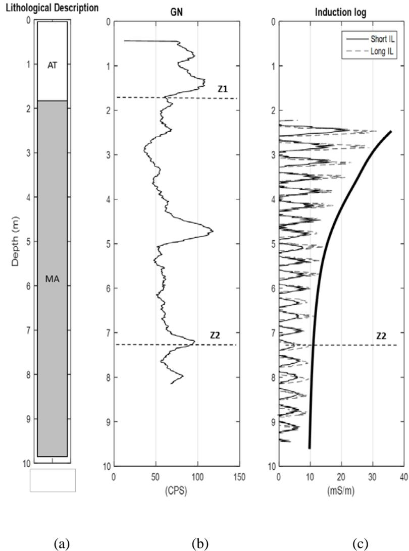
**Figure 6:** Induction and gamma-natural logging results: (a) lithological description, (b) gamma-natural profile in counts per second, and (c) induction-logging profiles in  $\text{mS}\cdot\text{m}^{-1}$ .
