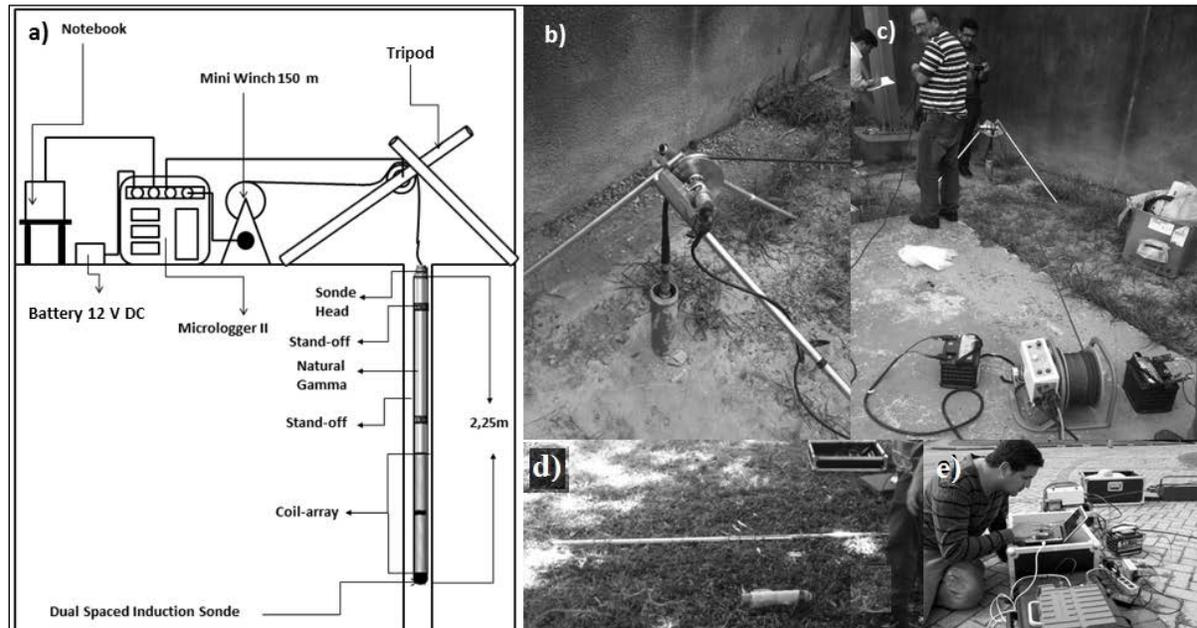
**Figure 5:** (a) General layout of the IL test equipment-(b) pulley and tripod, (c) mini winch 150 m and batteries, (d) dual spaced induction probe, and (e) micrologger connected to the notebook.
