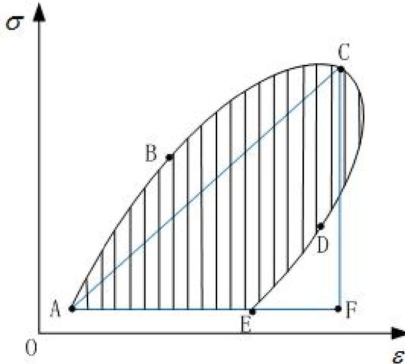
**Figure 9:** Determination of damping ratio
