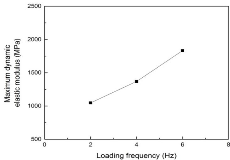
**Figure 14:** The relationship between maximum dynamic elastic modulus and loading frequency.
