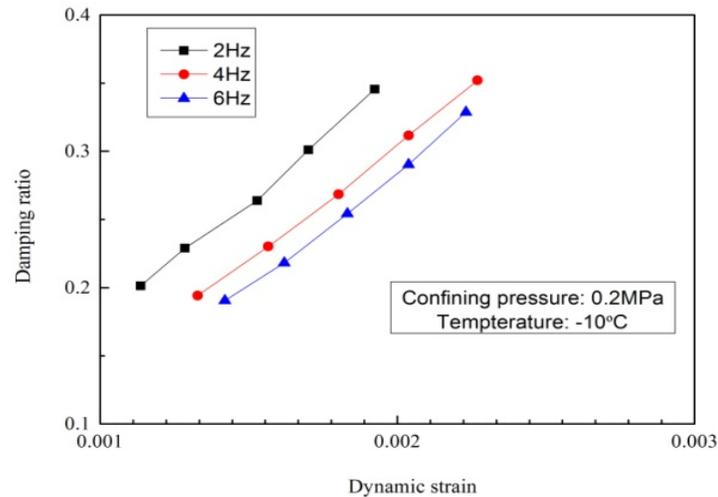
**Figure 15:** Damping ratios under different loading frequencies
