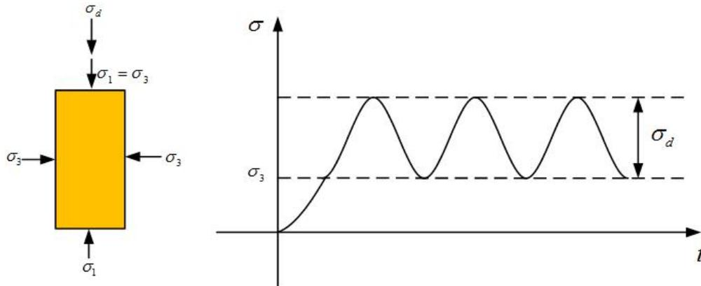
**Figure 7:** Load-on pattern of cyclic loading
