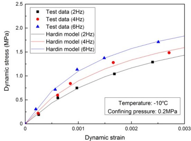
**Figure 13:** Backbone curves under different loading frequencies
