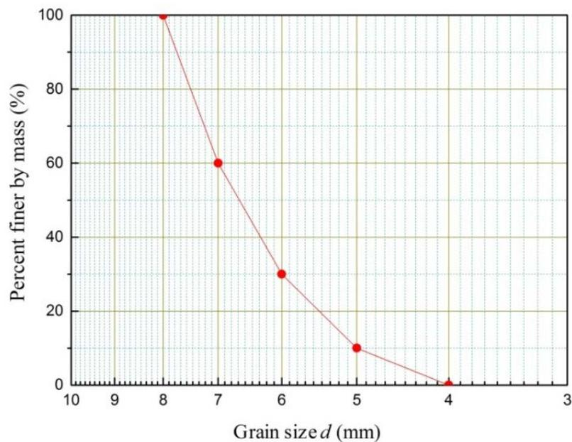
**Figure 2:** Grain size distribution curve of glass beads
