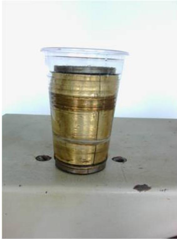
**Figure 4:** The specimen before freezing
