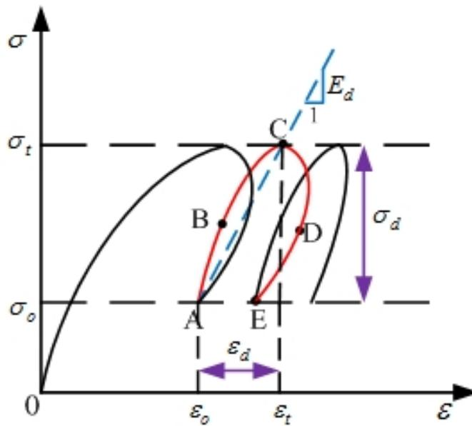
**Figure 8:** Determination of dynamic elastic modulus
