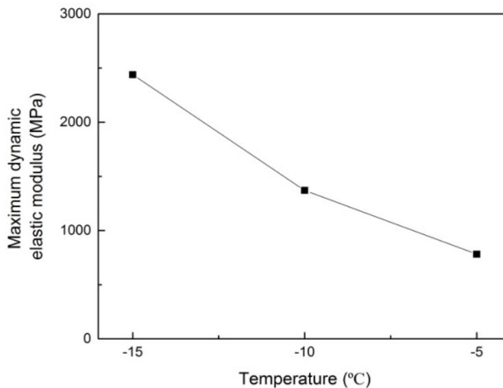
**Figure 11:** The relationship between maximum dynamic elastic modulus and temperature
