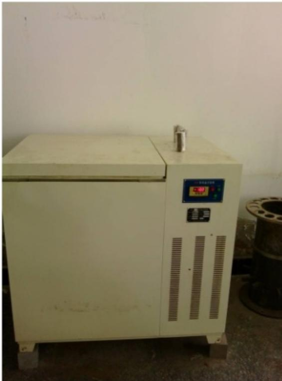
**Figure 5:** The automatic temperature-controlled refrigerator
