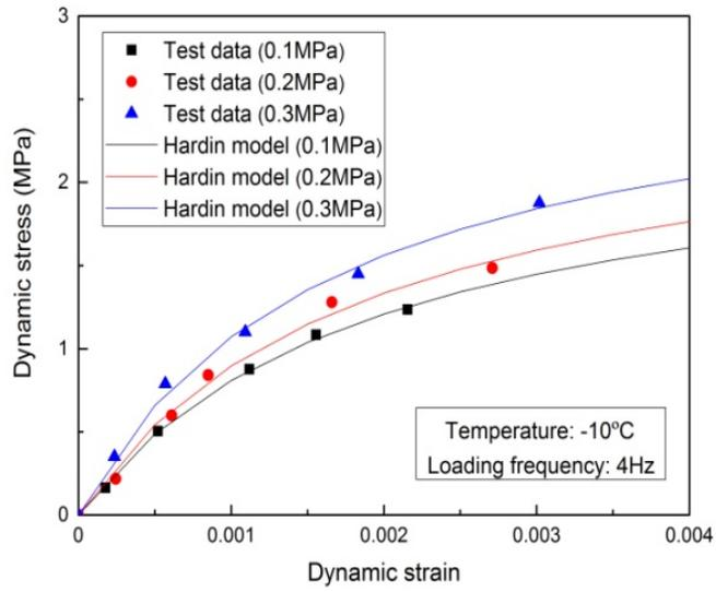
**Figure 16:** Backbone curves under different confining pressures
