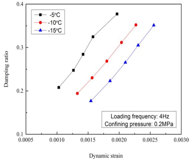
**Figure 12:** Damping ratios under different temperatures
