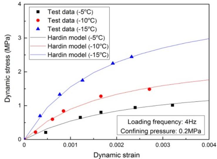
**Figure 10:** Backbone curves under different temperatures
