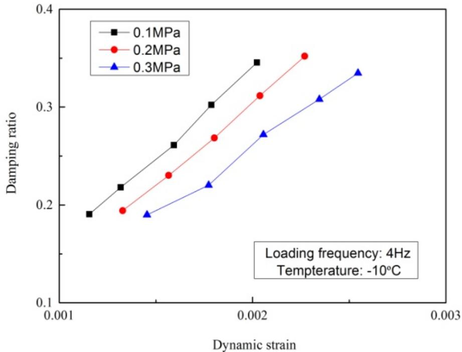
**Figure 18:** Damping ratios under different confining pressures
