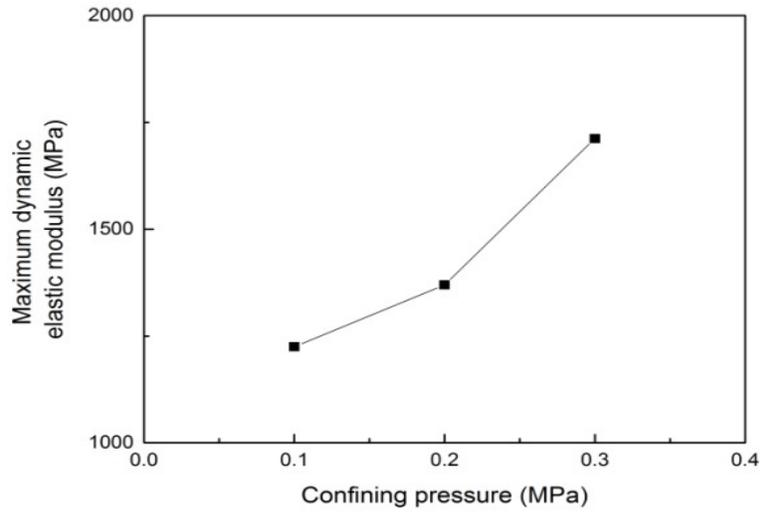
**Figure 17:** The relationship between maximum dynamic elastic modulus and confining pressure.
