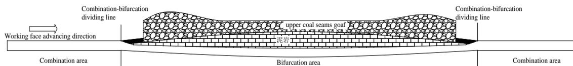
**Figure 1:** fully-mechanized continuous advancing method in BCCS
