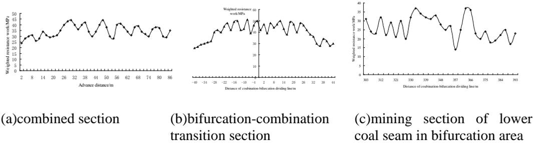
**Figure 6:** Resistance distribution of weighted support along the working face of different stages
