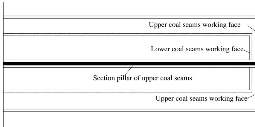
**Figure 2:** The staggered layout of upper and lower coal seam working face
