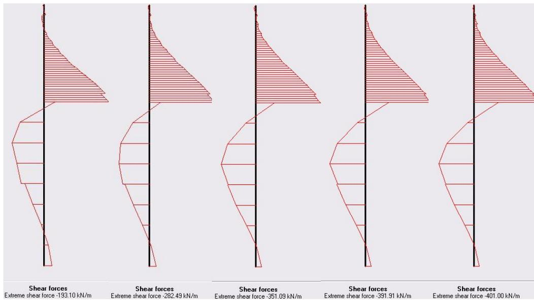
**Figure 7:** Distribution of shear force of each phase
