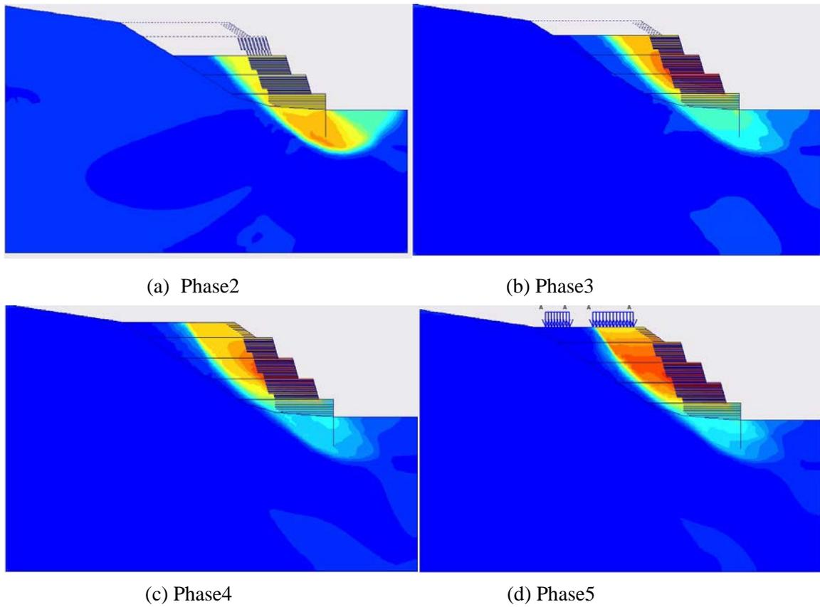
**Figure 5:** Potential failure surface of each phase
