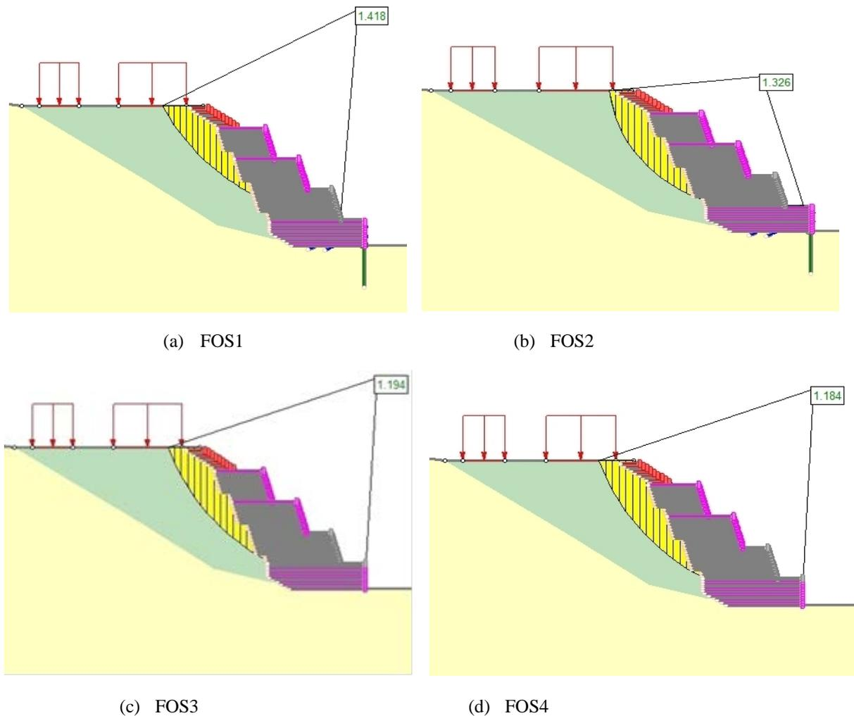
**Figure 2:** Potential failure surface calculated by Janbu simplified method
