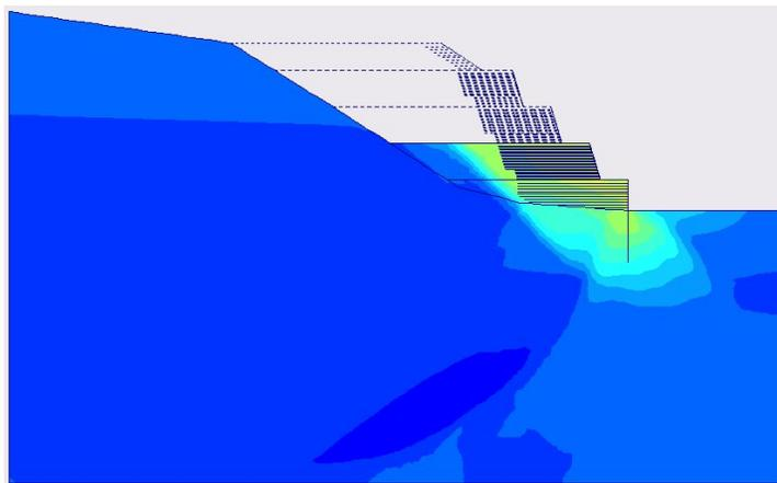
**Figure 4:** Potential failure surface of phase 1
