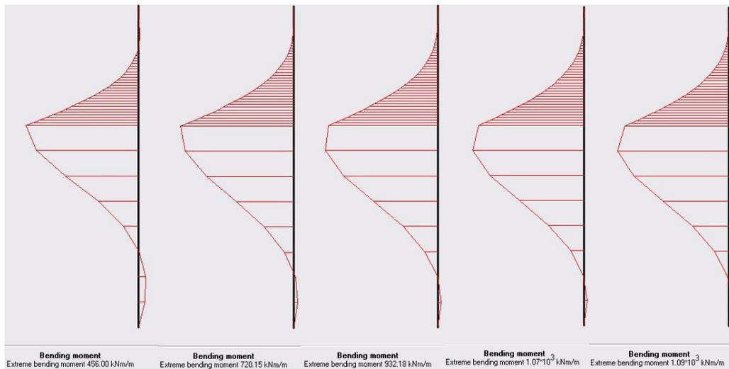
**Figure 6:** Distribution of bending moment of each phase
