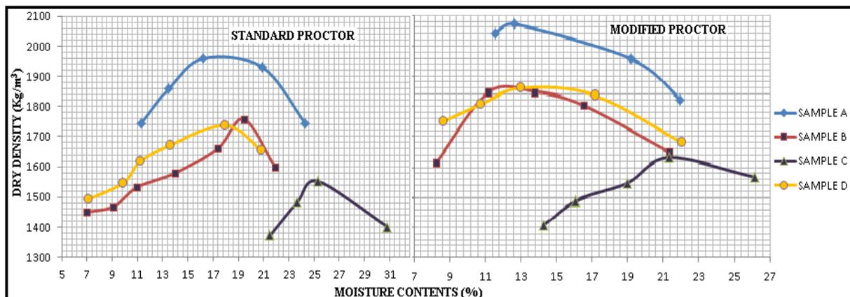
Figure 3: Compaction curves for the soil samples
