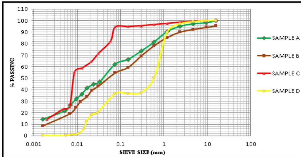
**Figure 2:** Particle Size Distribution curve of the samples
