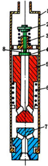
1-shell; 2-washer of movable valve seat; 3-valve spring; 4-movable valve;
