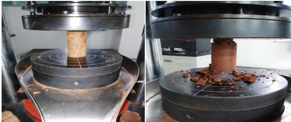
**Figure 3:** Cylinder rock uniaxial compressive test
