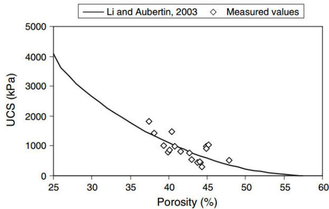
**Figure 8:** Comparison between the UCS values versus porosity predicted using Modified Li-Aubertin model and measured UCS values for the CPB samples solidified using three types of binders. (adapted from Ouellet, et al, 2008)
