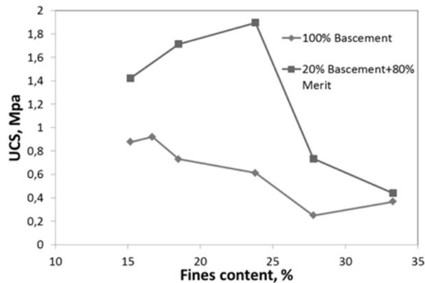
Figure 6 UCS variation as a function of fines contents in the CPB samples solidified by Bascement and mixture
