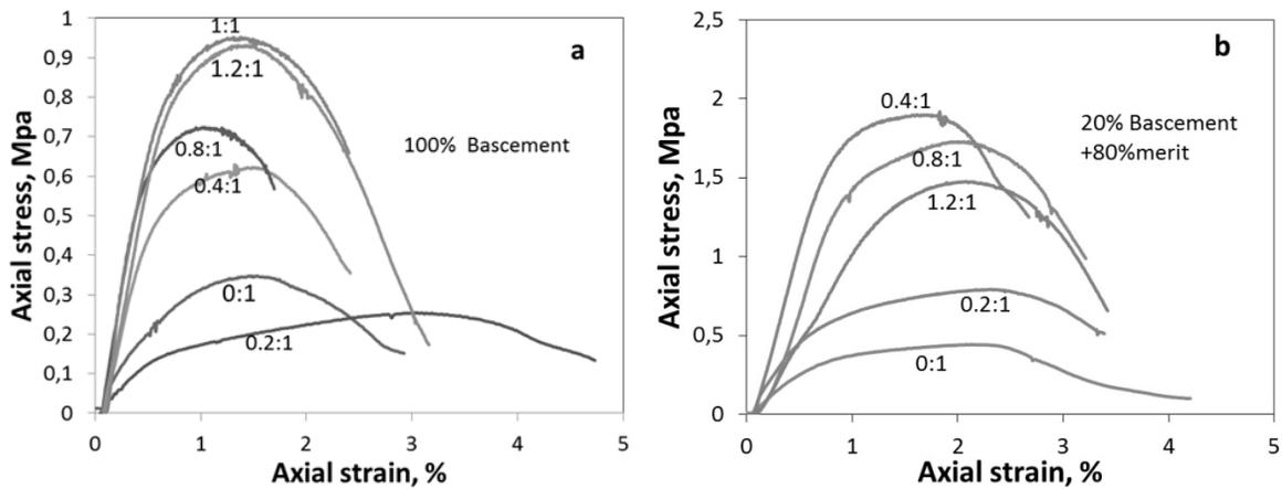
Figure 5 Uniaxial compression stress-strain relationships for (a) CPB samples using bascement as binder, (b) CPB samples using the mixture of 20% bascement+80% Merit as binder. The ratios shown on the curves are Fe-sand/tailings sand in dry weight
