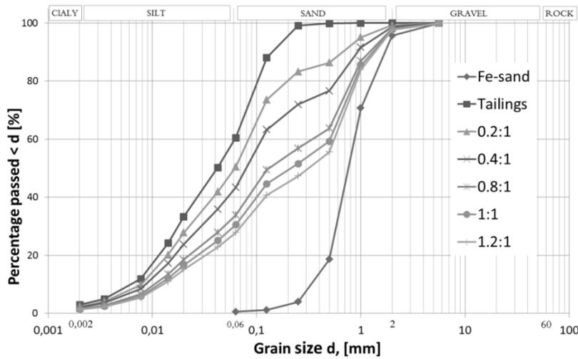
Figure 4 PSD, particle size distribution, of Fe-sand, the tailings sand and the CPB raw materials, mixtures of Fe-sand and tailings sand with dry-weight ratios of 0.2:1, 0.4:1, 0.8:1, 1:1 and 1.2:1
