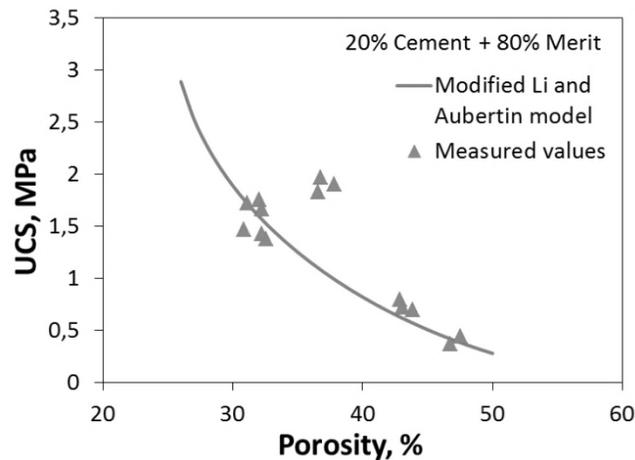
**Figure 10:** Comparison between the UCS values versus porosity predicted using Modified Li-Aubertin model and measured UCS values for the CPB samples solidified using mixture of 20% Bascement+80% Merit as binder in the present study.
