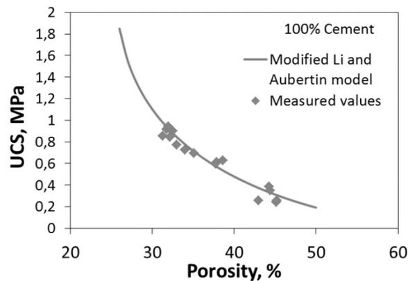
**Figure 9:** Comparison between the UCS values versus porosity predicted using Modified Li-Aubertin model and measured UCS values for the CPB samples solidified using bascement as binder in the present study.
