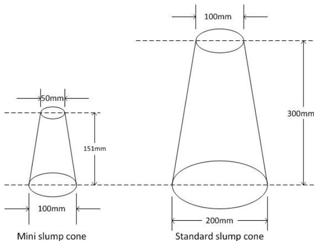
Figure 2 The dimensions of the mini slump cone and the standard slump cone
