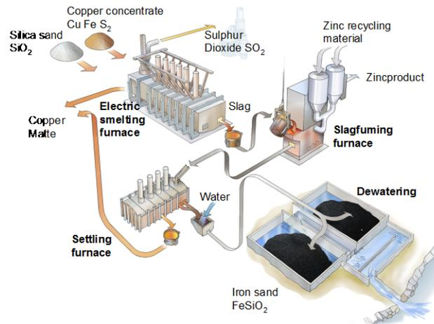
Figure 1. Process flow sheet of Cu settling furnace slag that is granulated to generate the Boliden Iron Sand
