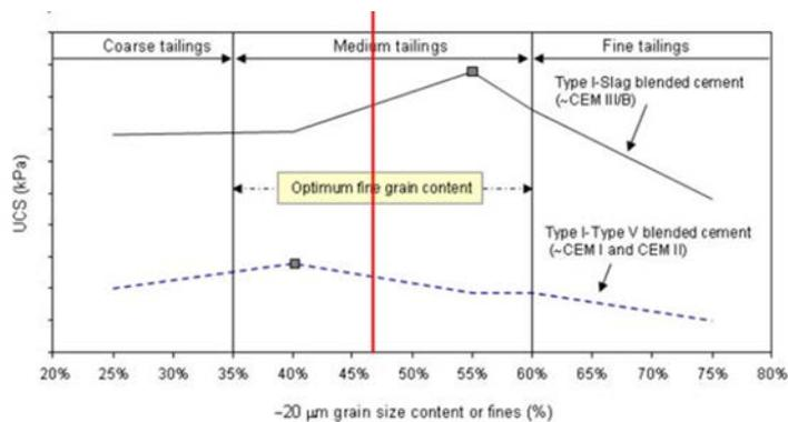
Figure 7 UCS variation as a function of fines contents in tailings solidified by two types of binders (adapted
