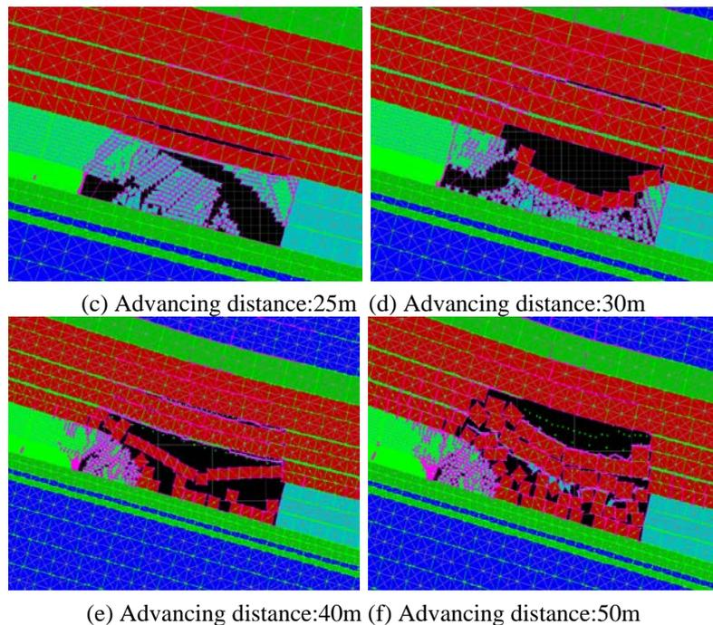
**Figure 2:** Movement law of overlying strata under different advancing distance
