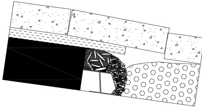
**Figure 4:** The roof mechanical model of an upward inclined top coal caving mining face
